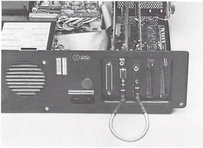
*Take the video cable and attach one of the female nine-pin sub mini D-type connectors into the lower nine-pin connector on the Quadlink end plate. Take the other end and connect it into the nine-pin connector on the video display card.*
