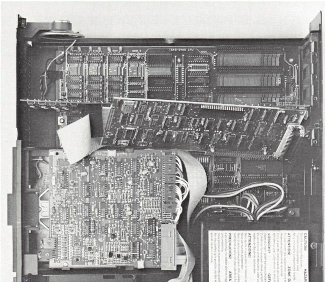
*Attach the Quadlink's disk controller cable to the left edge connector of the system's disk controller card. Again, make sure the pin line ups match as the connection is made. Then insert the disk controller card into expansion slot #5.*
