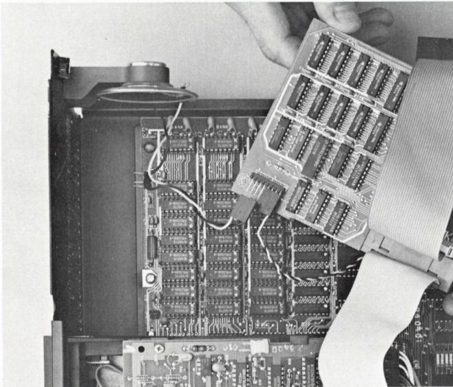
*Detach the speaker wire from the mother board connector and reroute the wire to connect it into the left-most gold pins located on the lower left corner of the board, next to the Quadlink's installed speaker wire.*
