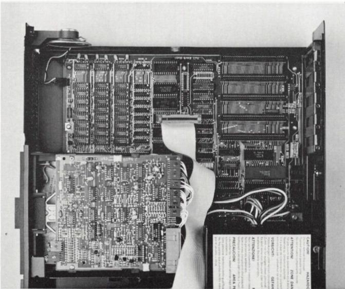
*To make room for installation of the Quadlink, remove all expansion cards from the system mother board and position the disk controller cable next to expansion slot #4. Now you are ready to begin.*
