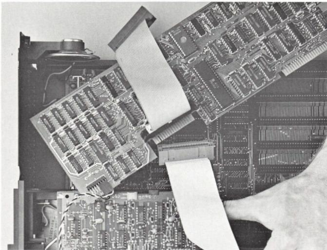
*Attach the disk controller cable into the lower rim of gold fingers located near the middle of the board. Make sure the connection is snug and the pin numbers on both connection points match.*
