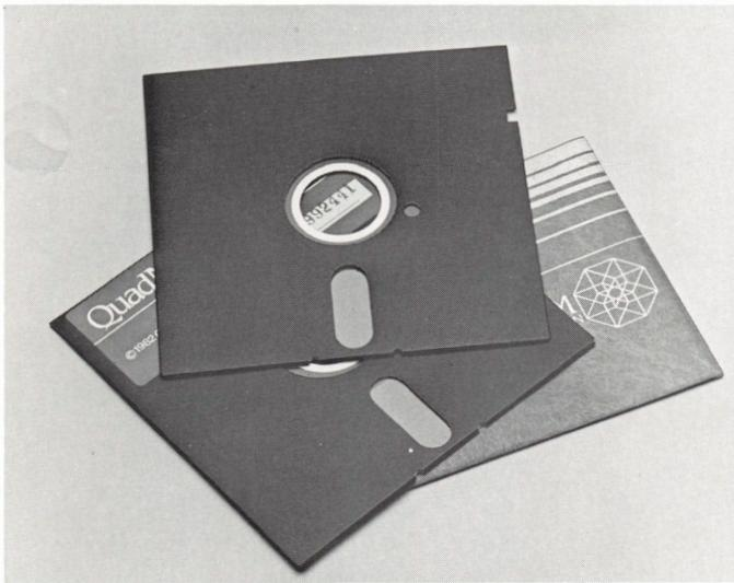
*Quadram's Quadlink with two software disks: one with the Quadlink's DOS and the other with a boot program.*
