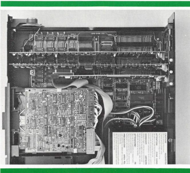
*The video display card can then be inserted into expansion slot #3 on the system board. And any other expansion card or Quadram enhancement board you are using can be inserted into the remaining slots at this point.*
