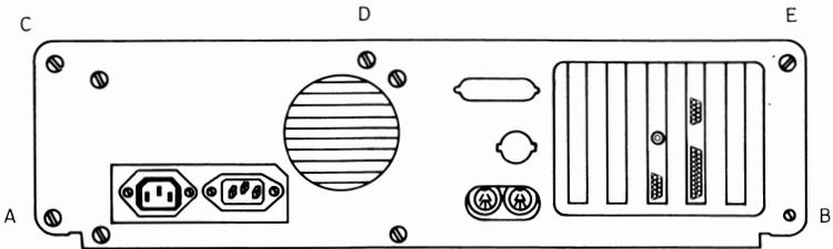
To open the computer the cover will have to be removed from the chassis. This is done by loosening two screws located at either end of the rear panel. These screws are marked A and B above: With your screwdriver, remove
