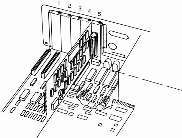
*The five expansion slots on the mother board are used to accommodate expansion cards.*
