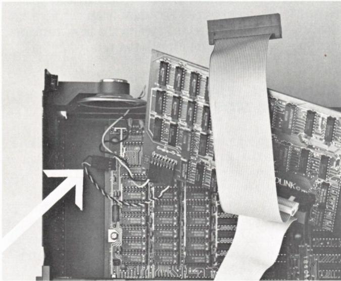
*Take the free end of the Quadlink's speaker wire and insert it into the mother board connector. When this is done the speaker will be wired through the Quadlink back to the mother board.*
