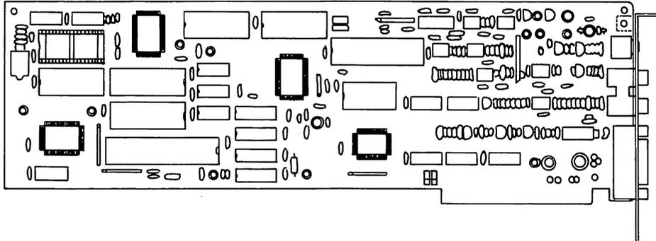
⑦ Align the card edge connector over the connector slot and push the LAPC-I board into the slot. Secure the board into the slot with the retaining screw.
