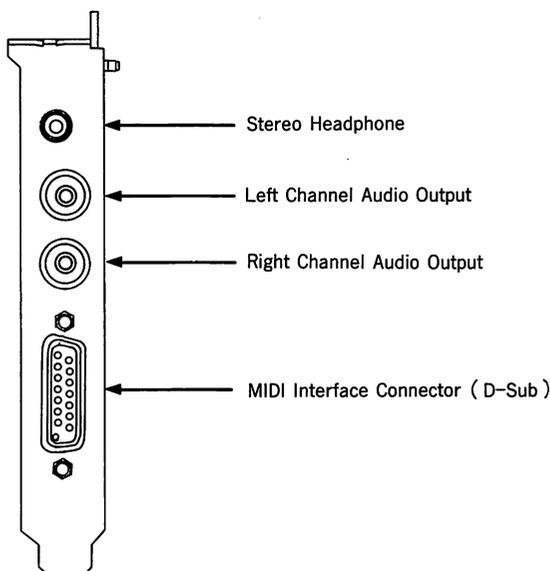
⑪ Connect the MIDI connector box MCB-1 to the MIDI interface Connector. This box provides the connectors for attaching MIDI equipped keyboards and other devices to the LAPC-I card. This box also contains a metronome beeper.
