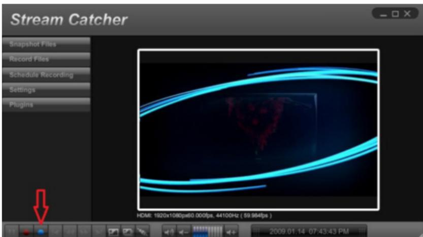
6. Using a different device on your network (Tablet, laptop, etc.) open the web browser and then type the full URL used in Step 5. The URL is built using your computer IP address with, “/live/session0.m3u8” added at the end.
