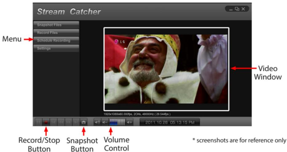
Manually recording video can be done by simply pressing the “Record” button from the control menu along the bottom of the Stream Catcher window. The frame around the video window will turn red while recording. When you would like to stop recording, press the “Stop” button. The “Snapshot” button allow you to take screen capture of the video stream.
