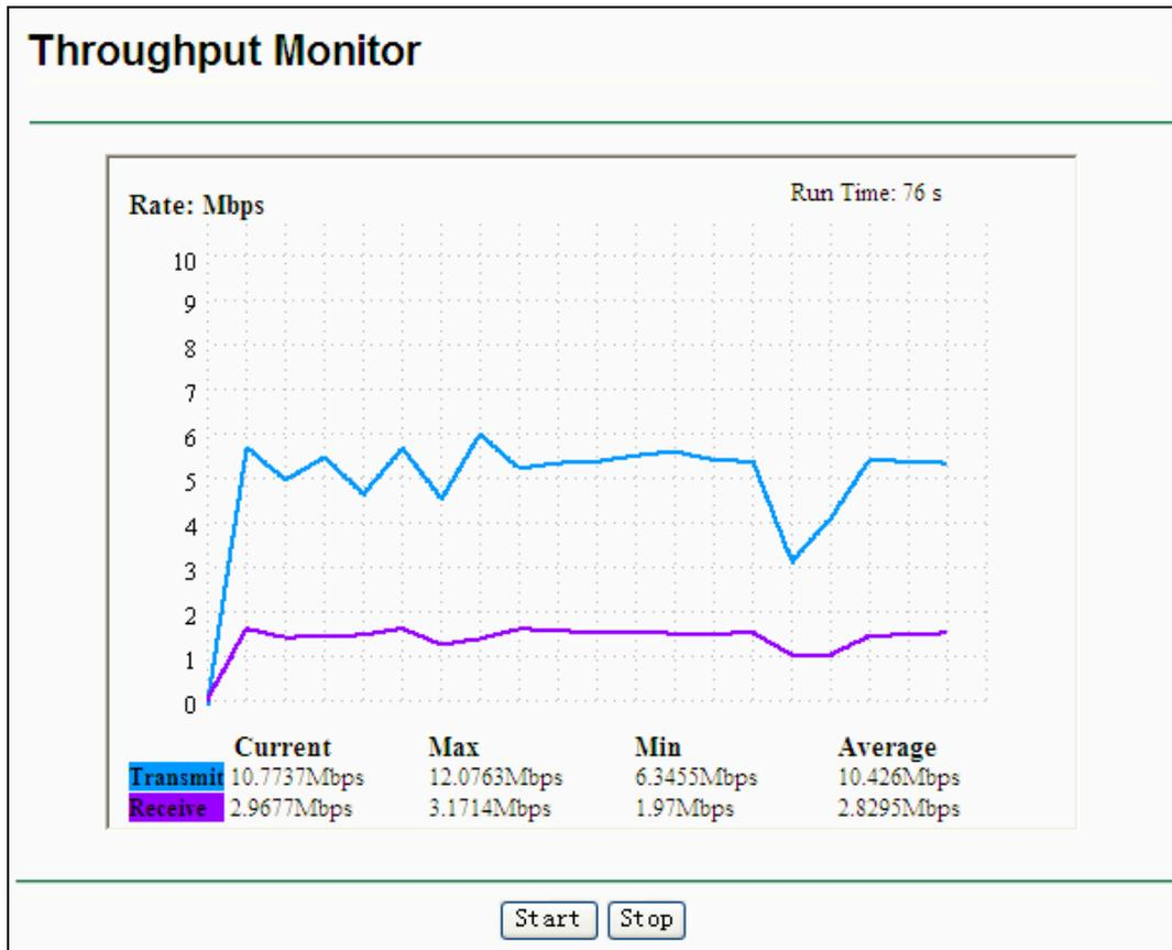
Figure 4-15 Throughput Monitor
