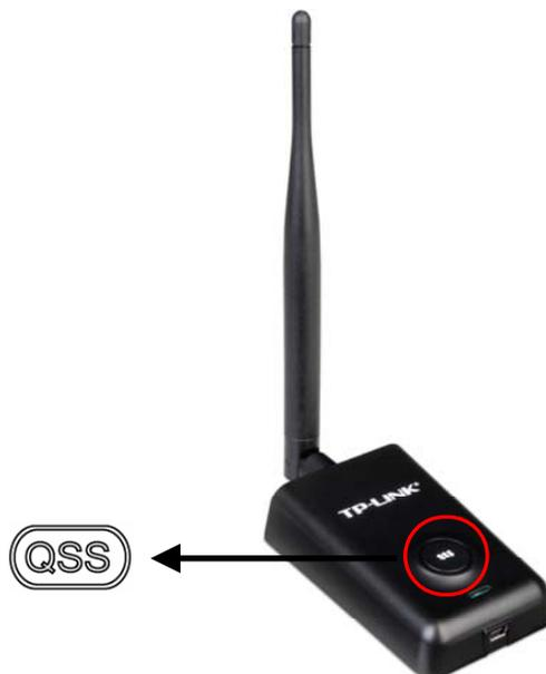
Step 2 Press the QSS button on your Access Point device to build the connection.
