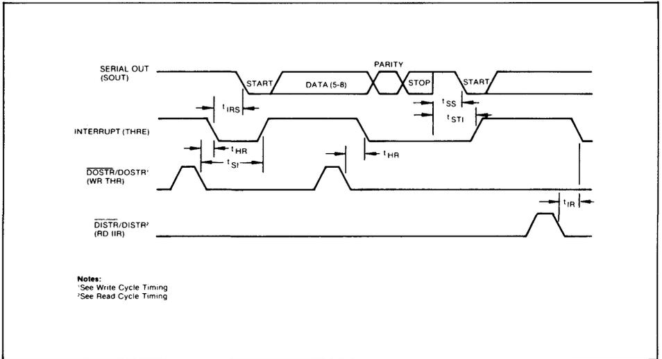
FIGURE 9. TRANSMITTER TIMING
