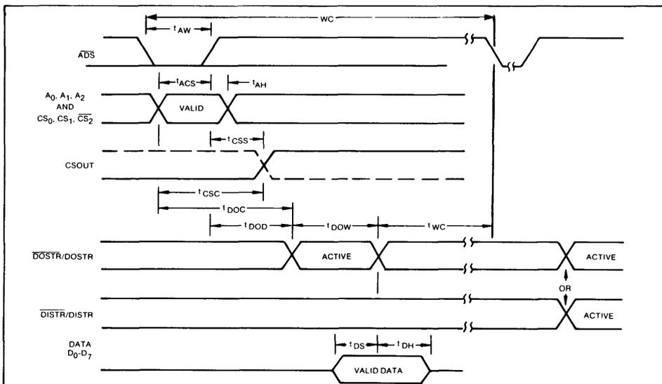
FIGURE 6. WRITE CYCLE TIMING
