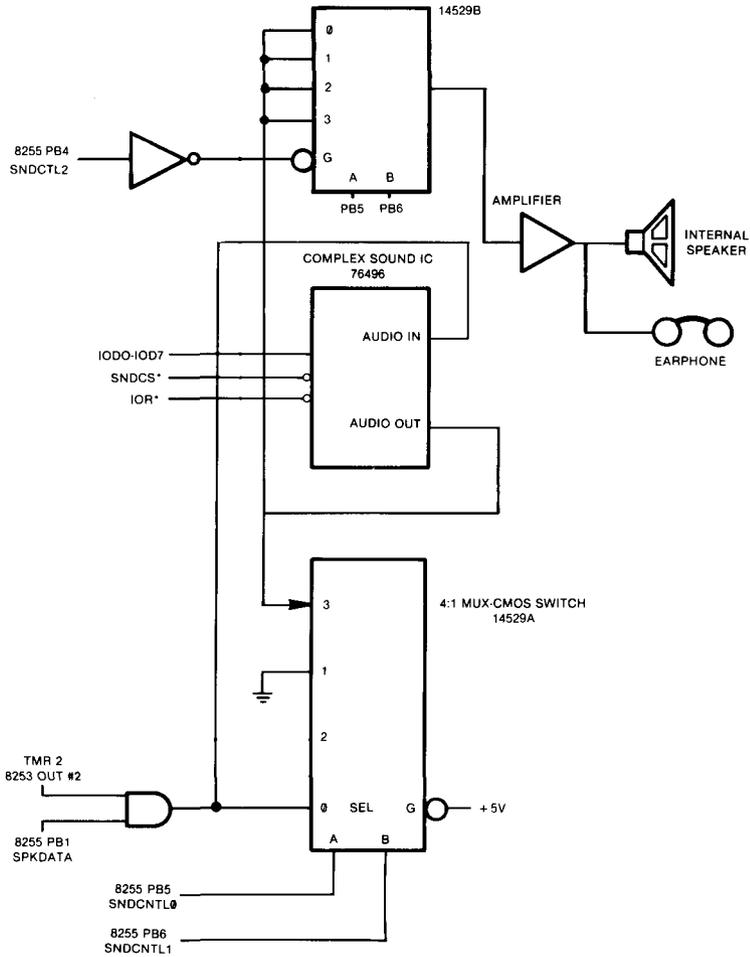
Figure 11. Sound Functional Block Diagram
