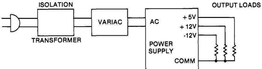
**Figure 1 Test Setup**
