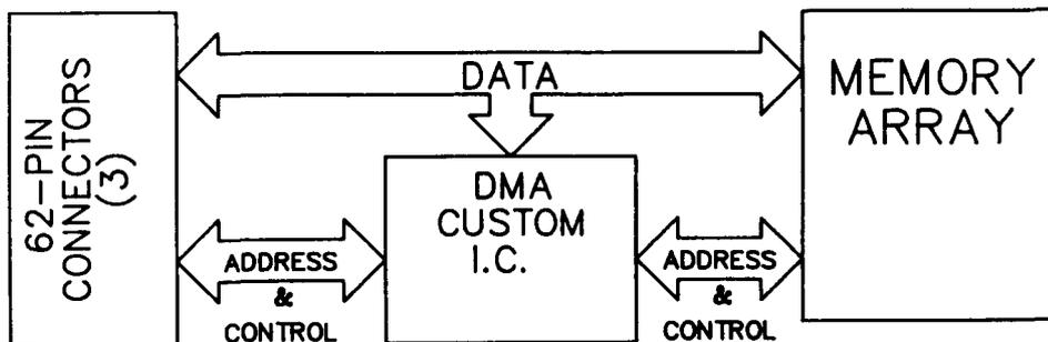
**Figure 1. Memory PLUS Expansion Adapter Block Diagram**
