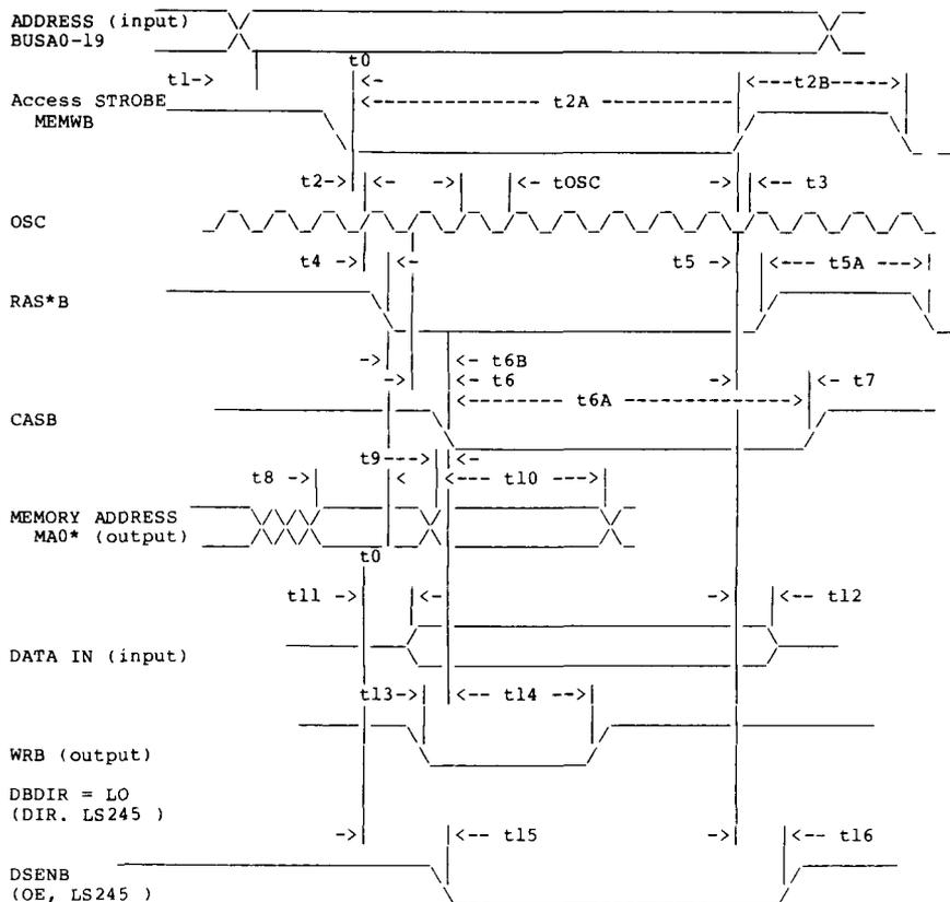
Figure 2. MEMORY TIMING PARAMETERS, WRITE
