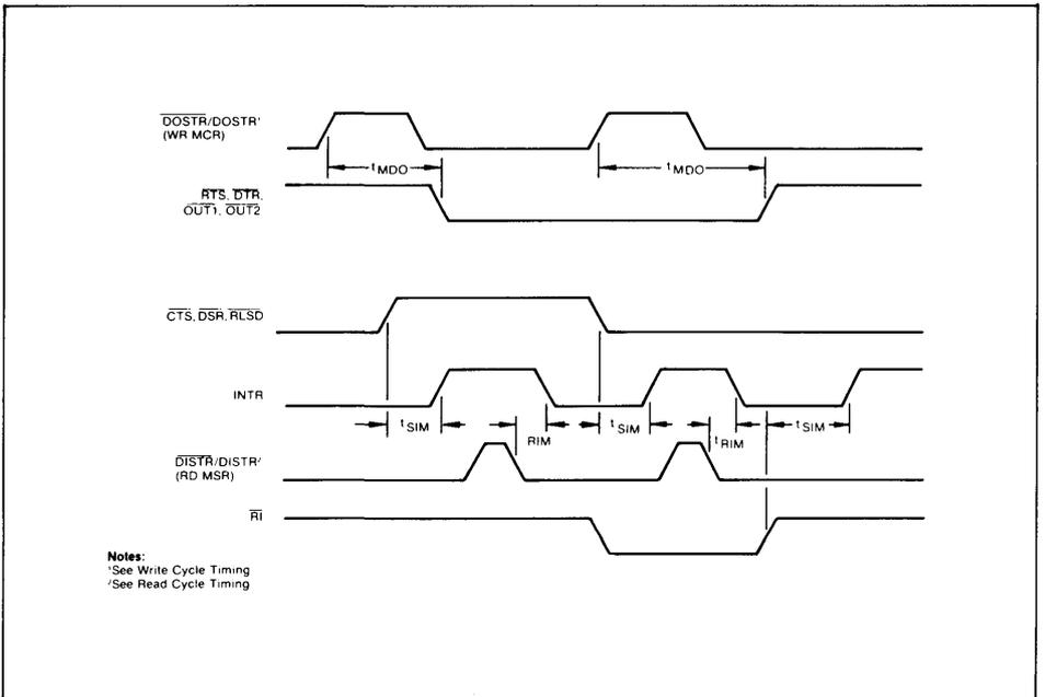
FIGURE 10. MODEM CONTROLS TIMING
