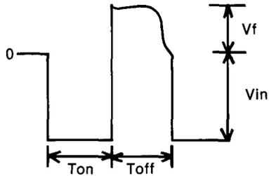
Collector Voltage Waveform
