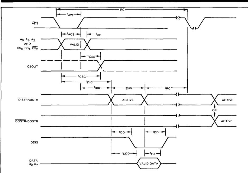
FIGURE 5. READ CYCLE TIMING
