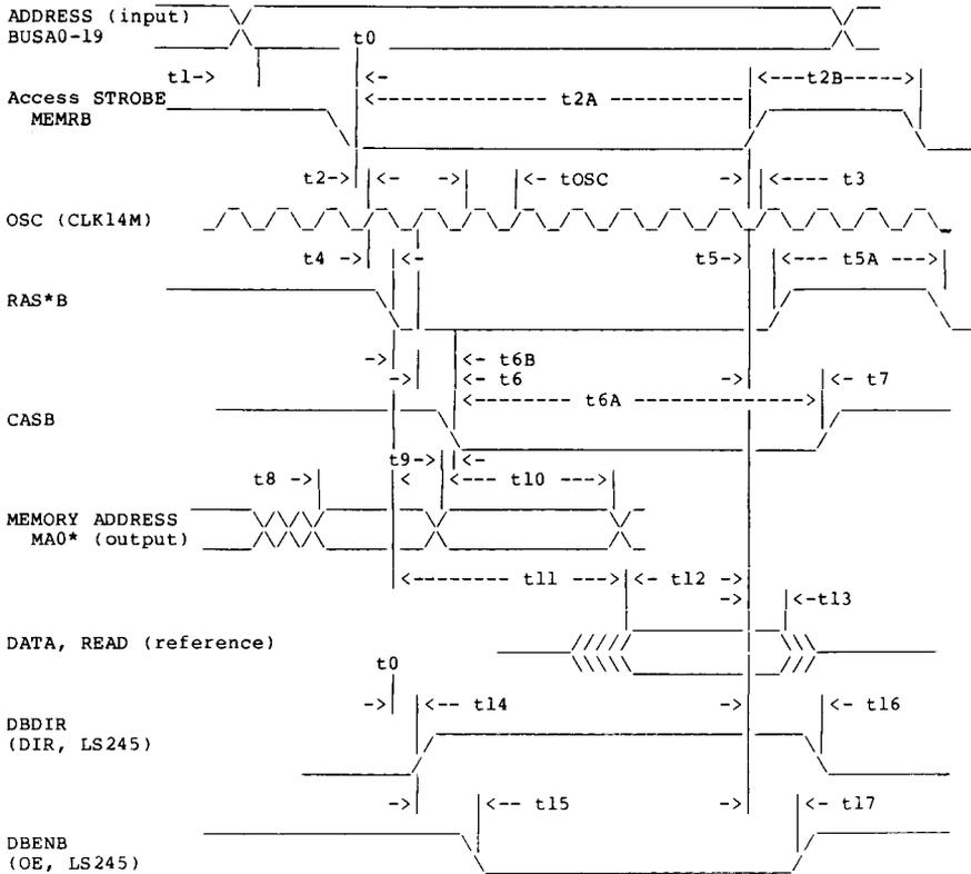
Figure 1. MEMORY TIMING PARAMETERS, READ
