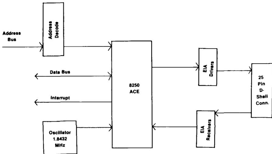
Figure 1. Block Diagram for the RS-232 Adapter.
