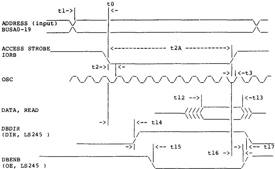
Figure 3. I/O CHIP SELECT PARAMETERS, READ
