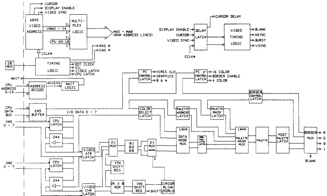
Figure 14. Video Controller Block Diagram
