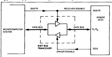
FIGURE 2. TYPICAL INTERFACE FOR A HIGH-CAPACITY DATA BUS.
