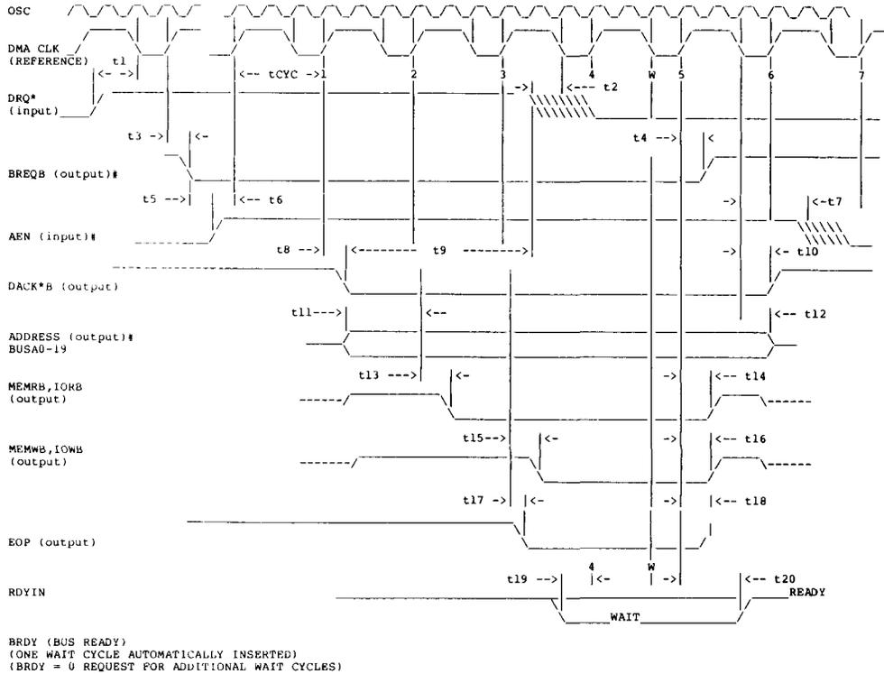
Figure 5. DMA BUS MASTER TIMING, READ / WRITE
