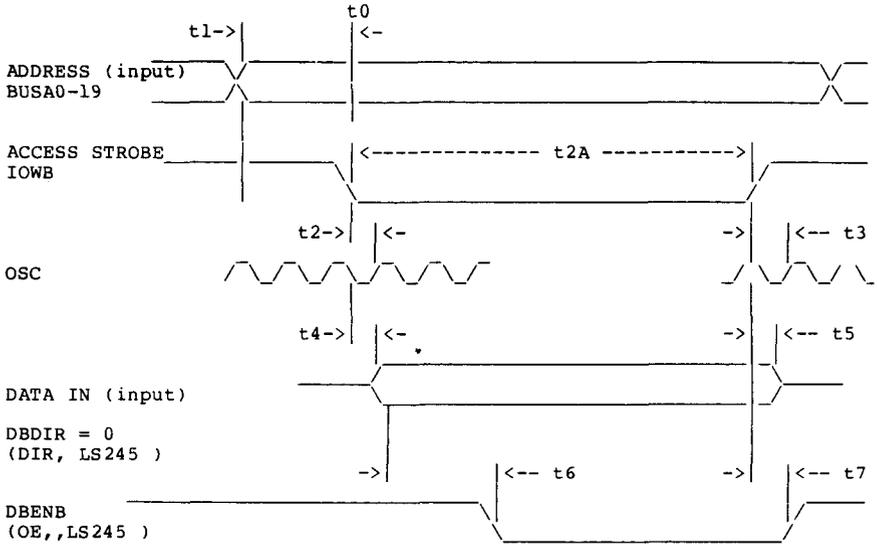
Figure 4. I/O CHIP SELECT PARAMETERS, WRITE
