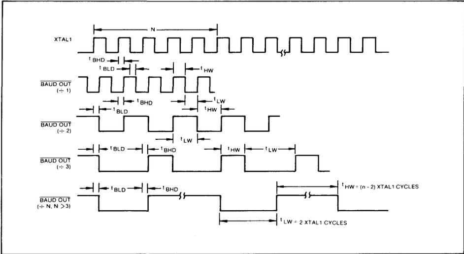
FIGURE 7. BAUDOUT TIMING
