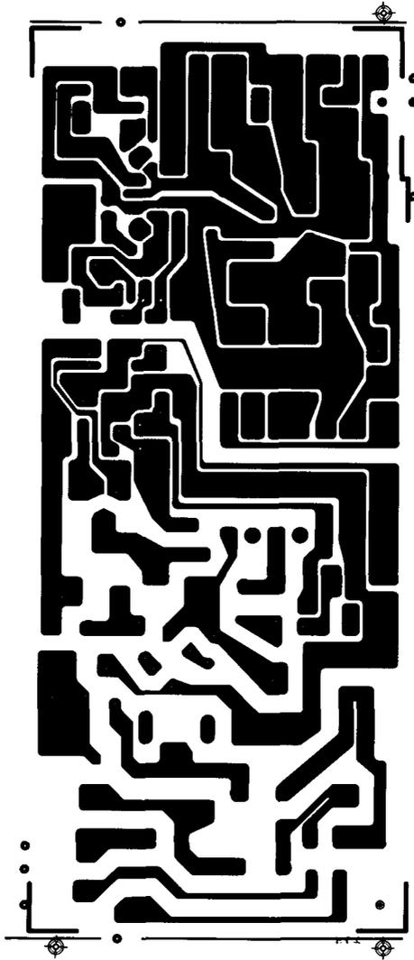
Power Supply PCB - Component Side
