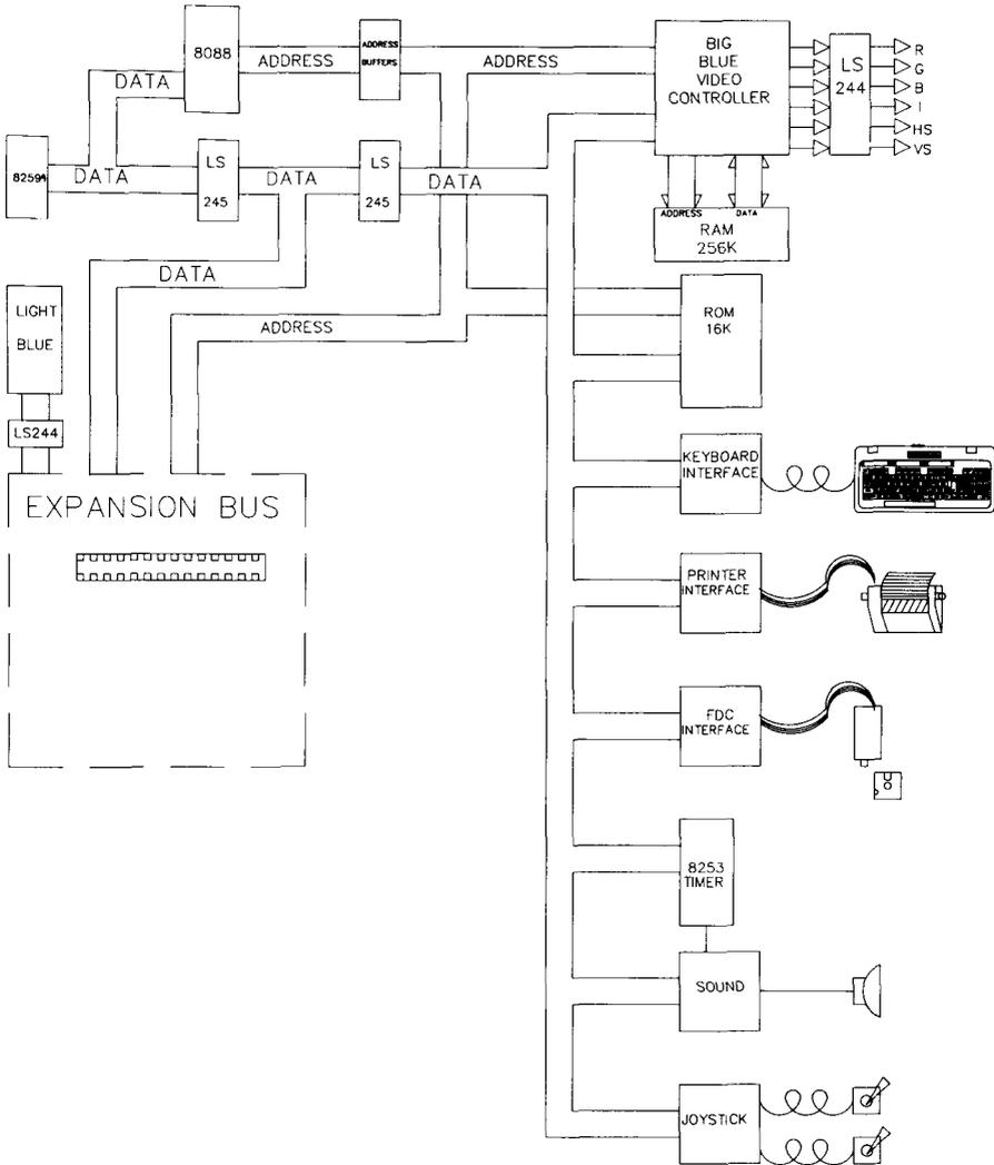
Figure 4. Main Logic Block Diagram
