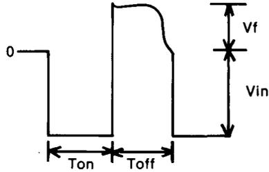
Collector Voltage Waveform
