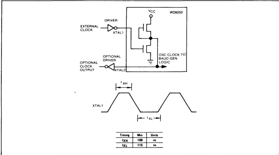
FIGURE 3. EXTERNAL CLOCK INPUT (3.1 MHz MAX.)
