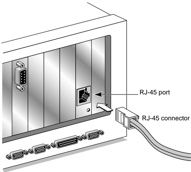
**Figure 2-2** Connecting the 3C509B-TPO NIC Using the RJ-45 Port
