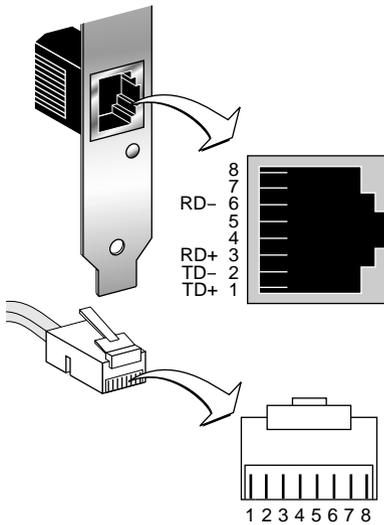
**Figure A-1** RJ-45 Connector Pin Assignments
