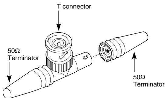
**Figure 5-1** Assembling a Loopback Plug
