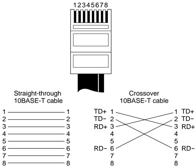
**Figure 5-2** Straight-through and Crossover Cable Pinouts
