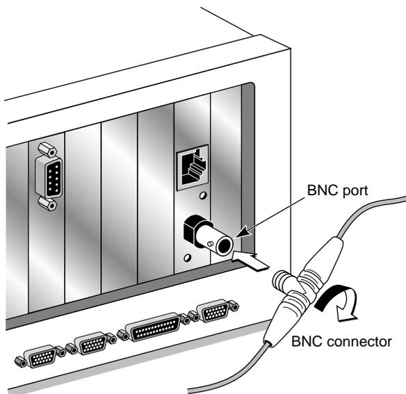
**Figure 2-3** Connecting the 3C509B-TPC NIC Using the BNC Port
