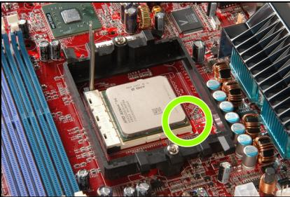
2. Align the corner with triangle mark of the processor with the marking on the motherboard, and then place the processor vertical down into the socket.
