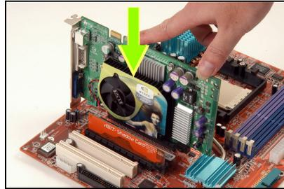
3. Insert a PCIE graphics card into PCIEXP1 slot.
