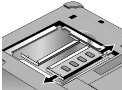
1. Release the two latches at the sides of the RAM expansion module by pushing them gently outward (away from the sides of the module). When you release the latches, the free edge of the module pops up.
