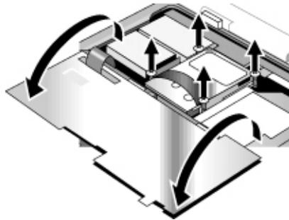
7. Unscrew the four Phillips-head screws from the sides of the hard disk drive case. (They remain attached to the case.)
