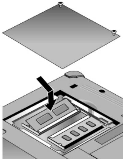
4. Insert the RAM expansion module into the connector at about a 30° angle until it's fully inserted. Then press down at both sides of the module until it latches.
