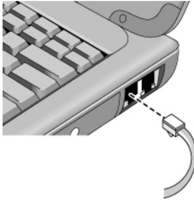
2. Plug the other end of the phone line into a telephone jack. (If the phone line does not fit your telephone jack, you may need to use an adapter.)
