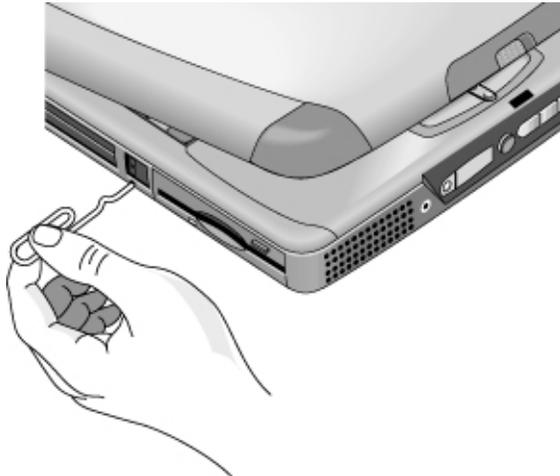
4. After the computer shuts down, slide the power switch and release it to turn the computer on again.
