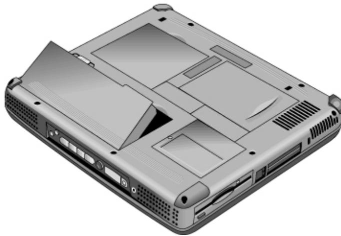
Once you have installed the battery, connect the AC adapter to the computer and recharge the battery while you work. You can also replace a low battery with another that is more fully charged.
