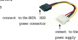
Please connect the black end of SATA power cable to the power connector on each drive. Then connect the white end of SATA power cable to the power connector of the power supply.
