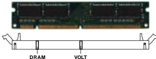
3. Close the plastic clip at the side of the DIMM slot.
