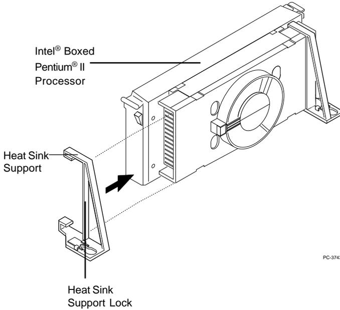
**Step 5:** Unlock the Processor Locks and Heat Sink Support Locks.
