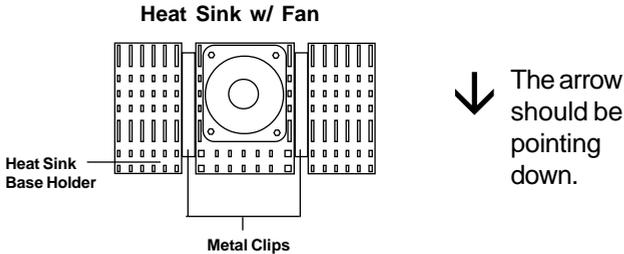
In case the metal clips are detached from the Heat Sink, re-attach them. Look for the arrow on the metal clip. This arrow should be pointing down and aligned with the Heat Sink Support Base Holder.
