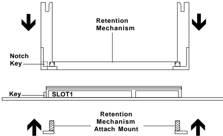
**Step 3:** Install the Heat Sink Support Base.
