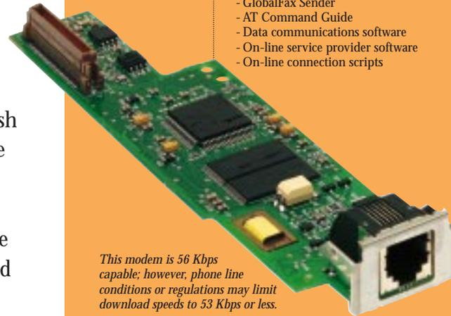
*This modem is 56 Kbps capable; however, phone line conditions or regulations may limit download speeds to 53 Kbps or less.*
