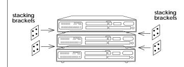
Use one pair of stacking brackets (included) for every BEN240 case you add to the stack. Each bracket comes with four holes (two for the lower case, two for the next case above). Attach the four included screws on one side and four on the other to secure the cases for vertical stacking.
