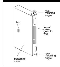
Use one pair of rack-mounting angles (included) for every BEN240 case you mount to the wall. Attach the 1 1/2" angle portion to two sides of the case using the provided screws. Attach the 7/8" angle portion to the wall. This will require 4 additional screws.
