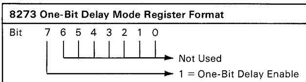
When one-bit delay is set, the 8273 retransmits the received data stream one-bit delayed. Reset of this bit stops the one-bit delay mode.
