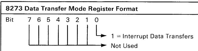
When the data transfer mode register is set, the 8273 protocol controller will interrupt when data bytes are required for transmission, or are available from a reception. If a transmit or receive interrupt occurs and the status register indicates that there is no transmit or receive interrupt result, the interrupt is a transmit or receive data request, respectively. Reset of this register causes DMA requests to be performed with no interrupts to the processor.
