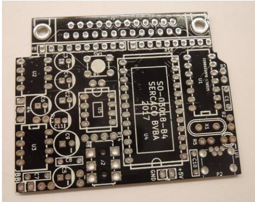
Starting from the blank PCB, gradually populate the board with components.
