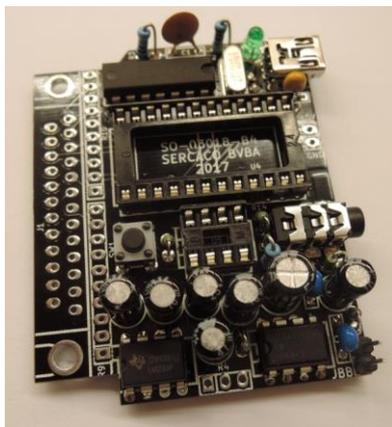
At this stage you can already test if the 5V power works fine : if there are no shorts , the green led should burn when you plug the board on an usb cable to your 5V power source. If this works, add the remaining components.
