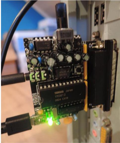
Now using the test program 'opl2test', you should hear some music. Adjust the potentiometer until you hear a suitable volume.
