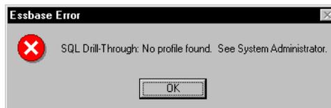
Figure 4-3, Essbase Error Message for Incomplete SQLDRILL.INI File
