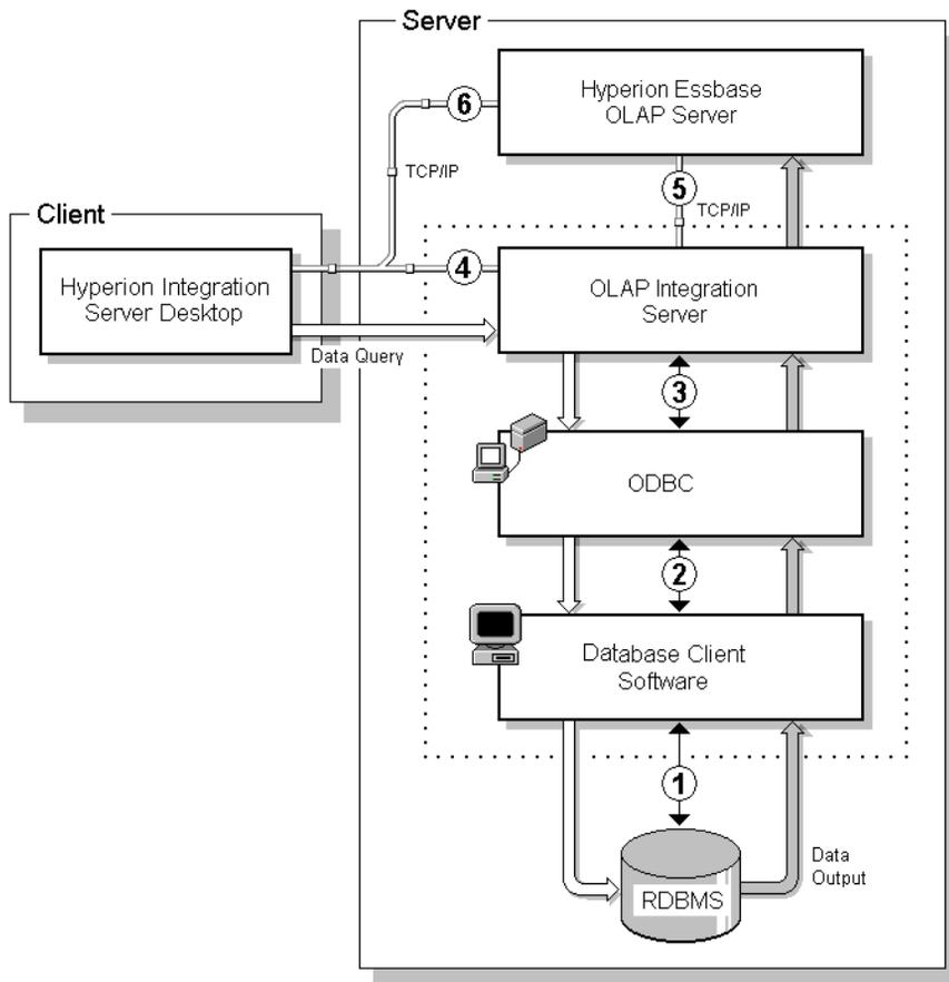
Figure 3-1: Hyperion Integration Server Components and Connections
