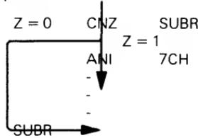
After the CNZ instruction has executed, if the Zero status does not equal 0 the ANI instruction will be executed. If the Zero status does equal 0, the address of the ANI instruction is saved at the top of the stack. The Stack Pointer is decremented by 2. The instruction labeled SUBR will be executed next.
