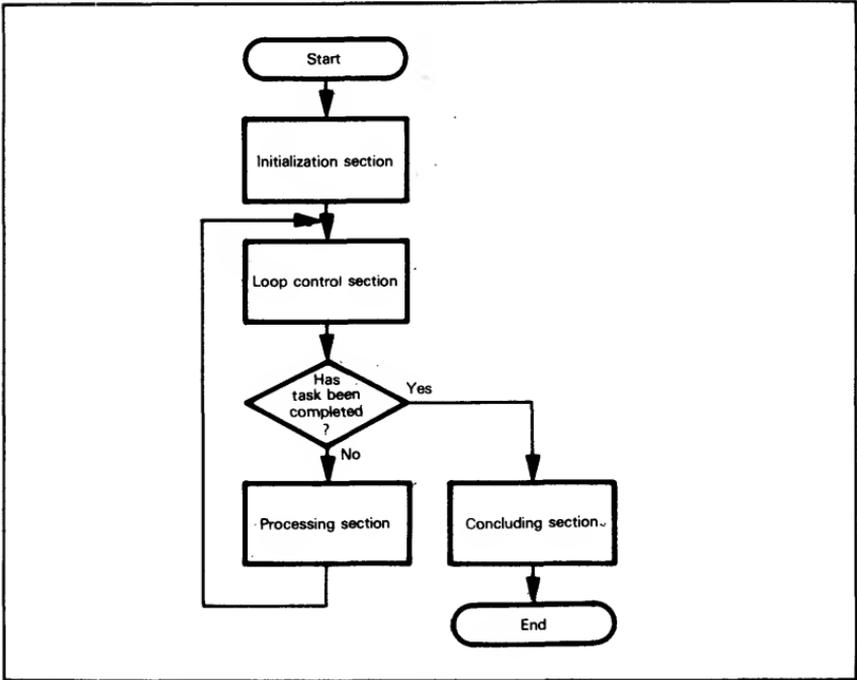
Figure 5-2. A Program Loop Which Allows Zero Iterations
