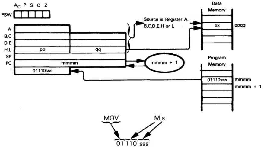
In either case, ddd or sss is interpreted as for a register-to-register move.
