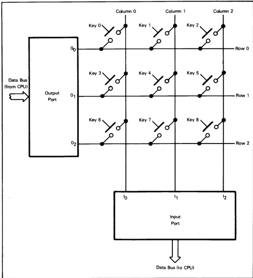
Figure 11-18. I/O Arrangement For A Keyboard Scan
