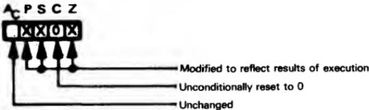
Within instruction execution illustrations, an X identifies a status that is set or reset. A 0 identifies a status that is always cleared. A blank means the status does not change.
