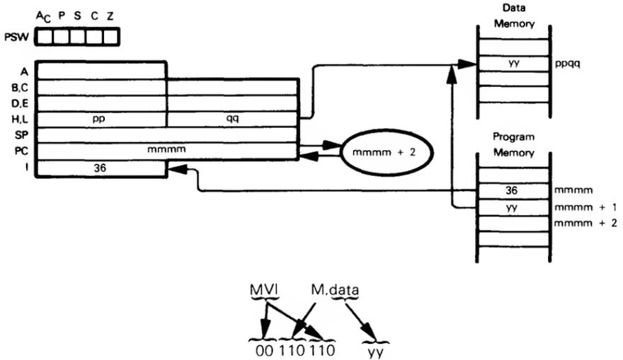
Suppose the H register contains  $03_{16}$  and the L register contains  $2A_{16}$ ; then when the instruction:
