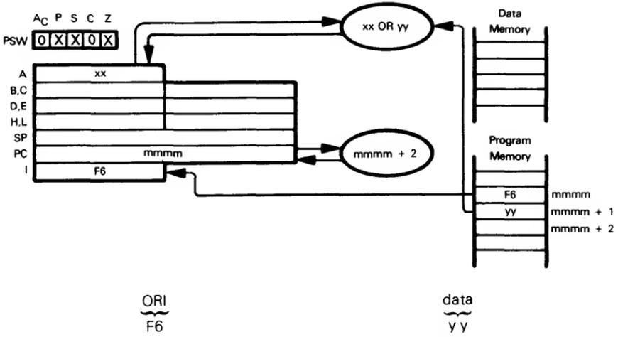
OR the Accumulator with the contents of the second instruction object code byte.
