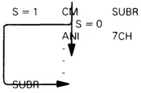
After the CM instruction has executed, if the Sign status does not equal 1 the ANI instruction will be executed. If the Sign status does equal 1, the address of the ANI instruction is saved at the top of the stack. The Stack Pointer is decremented by 2. The instruction labeled SUBR will be executed next.
