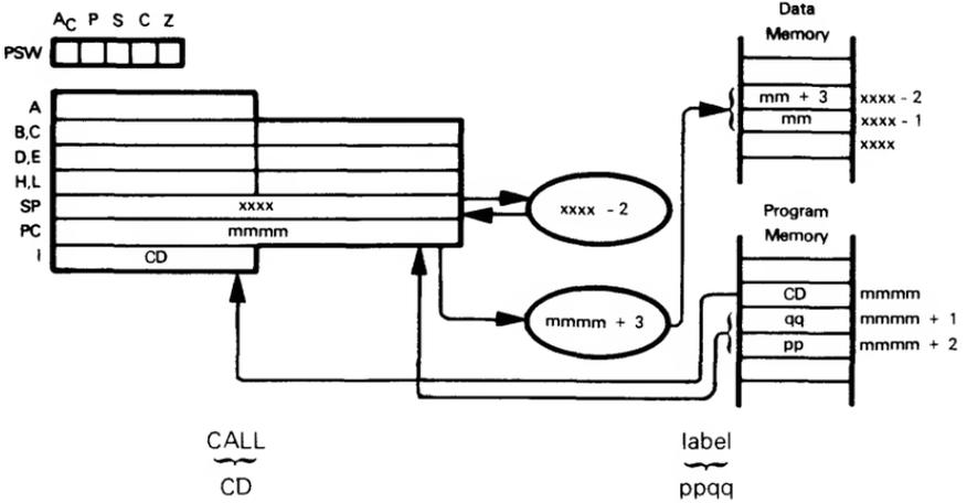
Store the address of the instruction following the CALL on the top of the stack; the top of the stack is a data memory byte addressed by the Stack Pointer. Then subtract 2 from the Stack Pointer in order to address the new top of stack. Move the 16-bit address contained in the second and third CALL instruction object program bytes to the Program Counter.
