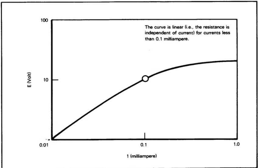
Figure 16-5. Typical E-I Curve for Thermistor (25°C)
