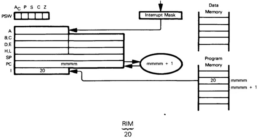
Load the contents of the restart interrupt mask and the serial input line into the Accumulator. The data loaded into the Accumulator is interpreted as follows:
