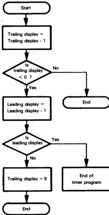
The value on the trailing display is decremented by 1. If this affects bit 4 (LEDON — used to turn the displays on), the value has become negative. A borrow must then be obtained from the leading display. If the borrow from the leading display affects bit 4, the count has gone past zero and the countdown is finished. Otherwise, the program sets the trailing display to '9' and continues.
