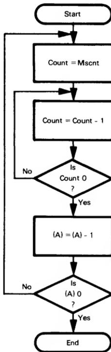
The value of MSCNT depends on the speed of the CPU and the memory cycle.
