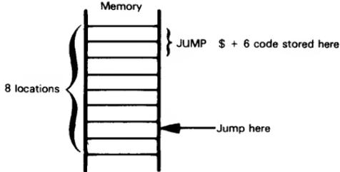
Most microprocessors have many two and three-word instructions. Thus you will have difficulty determining exactly how far apart two assembly language statements are. Therefore, using offsets from the Location Counter frequently results in errors which you can avoid if you use labels.
