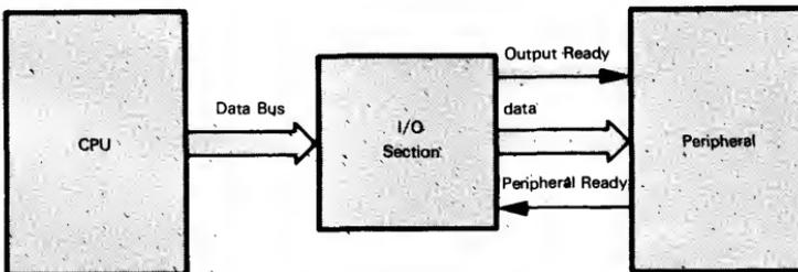
d) CPU sends Output Ready signal to Peripheral (this may be a hardware connection).
