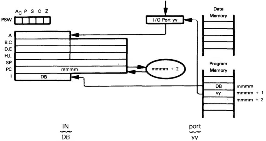
Load a byte of data into the Accumulator from the I/O port identified by the second IN instruction object code byte.
