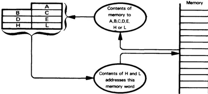
A limited number of instructions use Registers B and C, or D and E as the Data Pointer. These instructions move data between the Accumulator and the memory location addressed by Registers B and C or Registers D and E.
