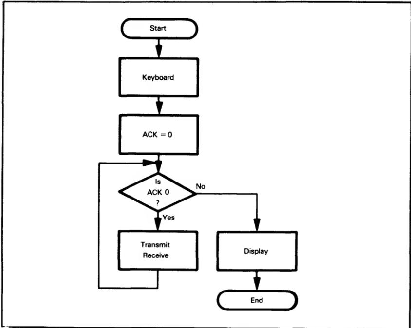
Figure 13-17. Initial Flowchart For Transaction Terminal
