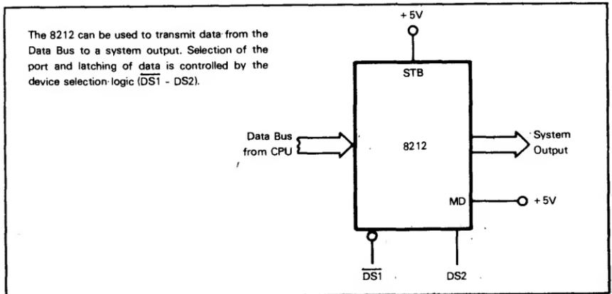
Figure 11-24. The 8212 I/O Port As A Latched Output Port
