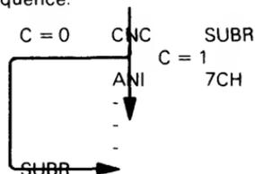
After the CNC instruction has executed, if the Carry status does not equal 0 the ANI instruction will be executed. If the Carry status does equal 0, the address of the ANI instruction is saved at the top of the stack. The Stack Pointer is decremented by 2. The instruction labeled SUBR will be executed next.
