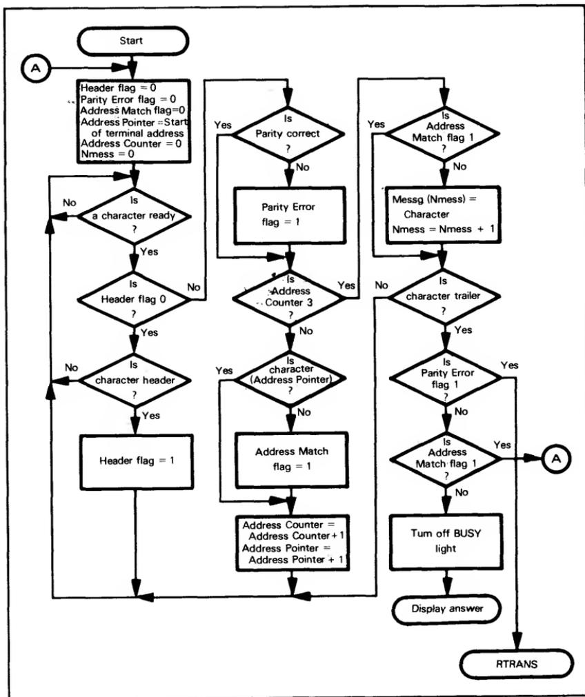
Figure 13-13. Flowchart Of Receive Routine
