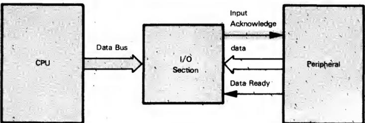
d) CPU sends Input Acknowledge signal to I/O section which then provides Input Acknowledge signal to Peripheral (this may be a hardware connection).
