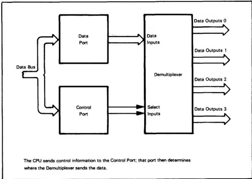
Figure 11-2. An Output Demultiplexer Controlled By A Port
