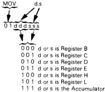
Move the contents of any register to any register. For example:
