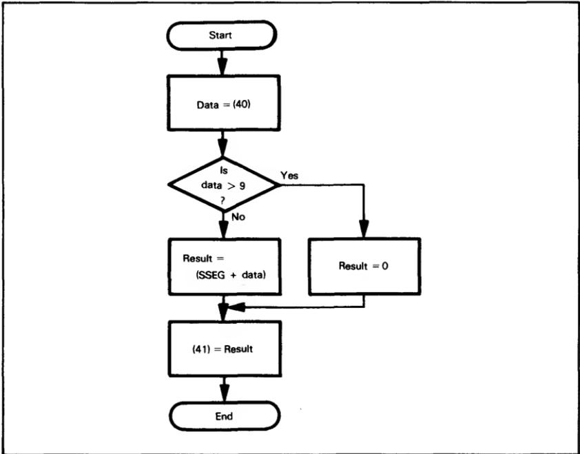
Figure 14-5. Flowchart Of Decimal To 7-Segment Conversion
