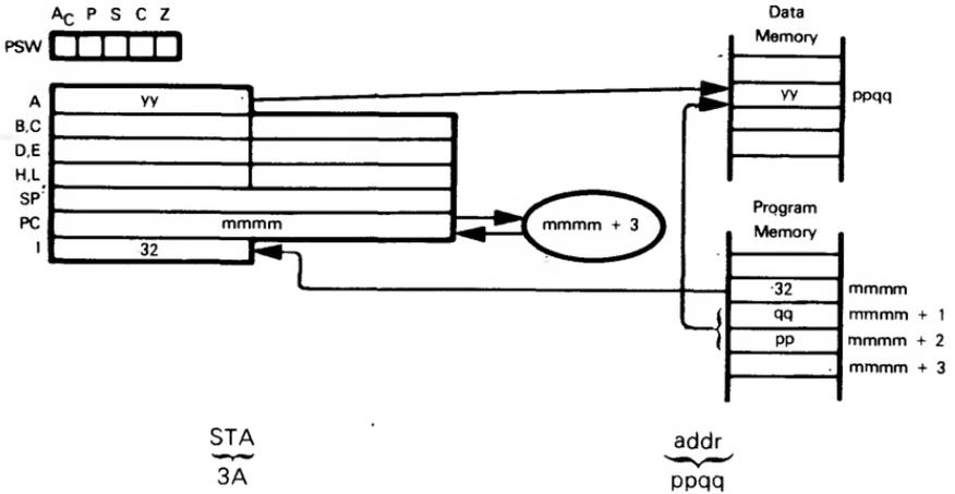
Store the Accumulator contents in the memory byte addressed directly by the second and third bytes of the STA instruction object code.
