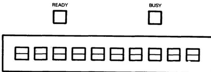
The display consists of ten 7-segment displays, which may be multiplexed, controlled by a shift register, or addressed separately. Two additional lights, READY and BUSY, are also present.
