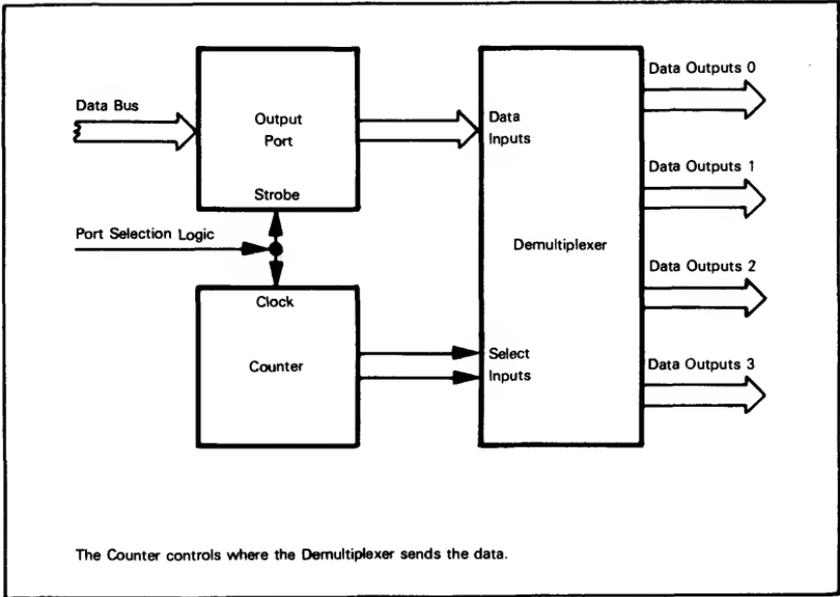
Figure 11-1. An Output Demultiplexer Controlled By A Counter
