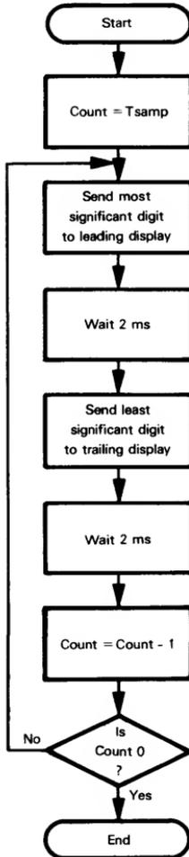
Each display is pulsed often enough so that it appears to be lit continuously. If TPULS were made longer (say 50 ms), the displays would appear to flash on and off.
