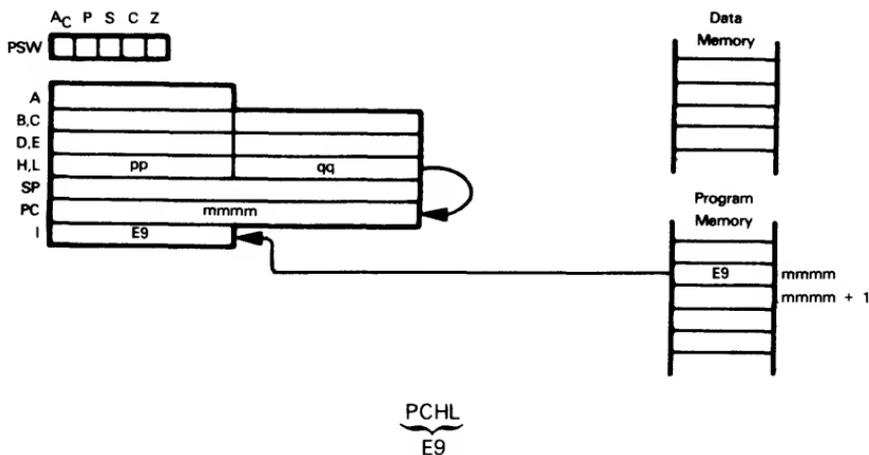
The contents of the H and L registers are moved to the Program Counter; therefore an implied addressing jump is performed.
