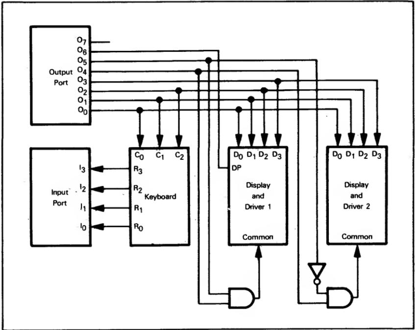
Figure 16-1. I/O Configuration
