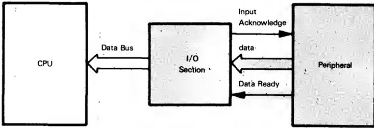
a) Peripheral provides data and Data Ready signal to computer I/O section.
