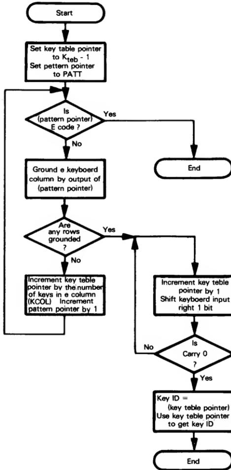
The particular key closed is identified by grounding single columns and observing whether a closure is found. Once a closure is found (so the key column is known), the key row can be determined by shifting the input.
