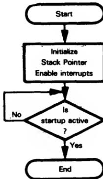
Note that hardware rather than software determines whether the startup is active.
