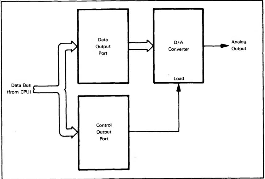
Figure 11-23. Interface For An 8-Bit Digital-To-Analog Converter
