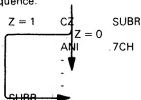
After the CZ instruction has executed, if the Zero status does not equal 1 the ANI instruction will be executed. If the Zero status does equal 1, the address of the ANI instruction is saved at the top of the stack. The Stack Pointer is decremented by 2. The instruction labeled SUBR will be executed next.
