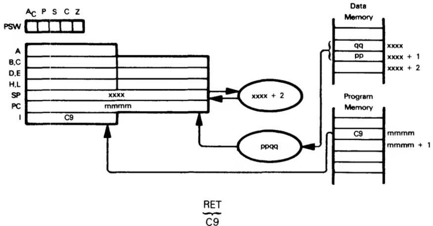
Move the contents of the top two stack bytes to the Program Counter; these two bytes provide the address of the next instruction to be executed. Previous Program Counter contents are lost. Increment the Stack Pointer by 2 to address the new top of stack.
