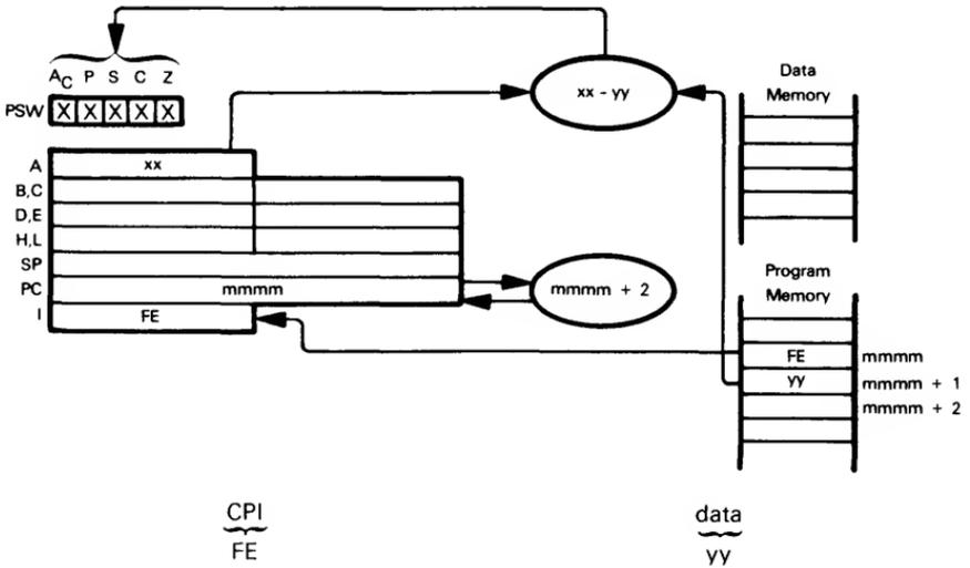
Subtract the contents of the second object code byte from the contents of the Accumulator, treating both numbers as simple, binary data. Discard the result, i.e., leave the Accumulator alone, but modify the status flags to reflect the result of the subtraction.
