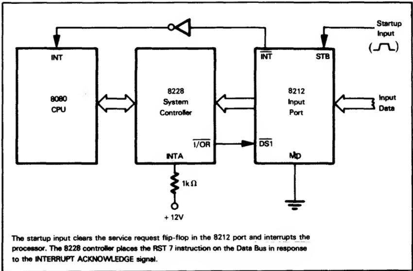
Figure 12-8. A Single Input Interrupt
