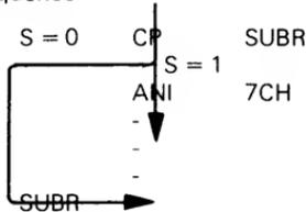
After the CP instruction has executed, if the Sign status does not equal 0 the ANI instruction will be executed. If the Sign status does equal 0, the address of the ANI instruction is saved at the top of the stack. The Stack Pointer is decremented by 2. The instruction labeled SUBR will be executed next.
