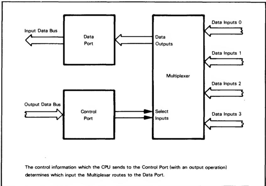
Figure 11-4. An Input Multiplexer Controlled By A Port
