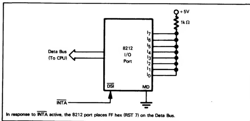
Figure 12-3. Using an 8212 I/O Port to Form the RST 7 Instruction
