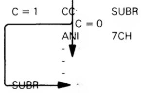
After the CC instruction has executed, if the Carry status does not equal 1 the ANI instruction will be executed. If the Carry status does equal 1, the address of the ANI instruction is saved at the top of the stack. The Stack Pointer is decremented by 2. The instruction labeled SUBR will be executed next.
