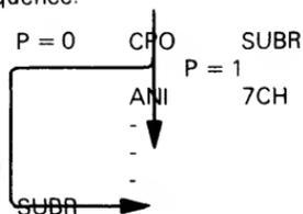
After the CPO instruction has executed, if the Parity status does not equal 0 the ANI instruction will be executed. If the Parity status does equal 0, the address of the ANI instruction is saved at the top of the stack. The Stack Pointer is decremented by 2. The instruction labeled SUBR will be executed next.
