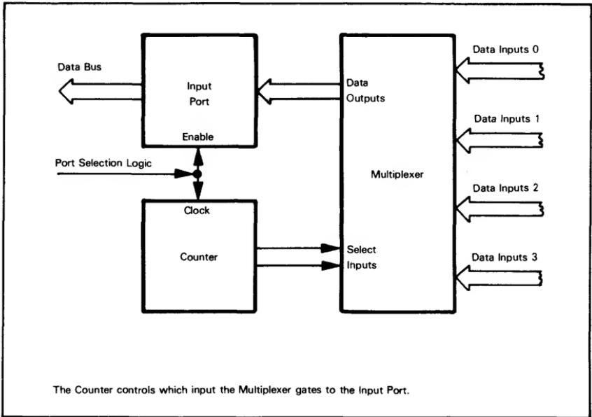
Figure 11-3. An Input Multiplexer Controlled By A Counter
