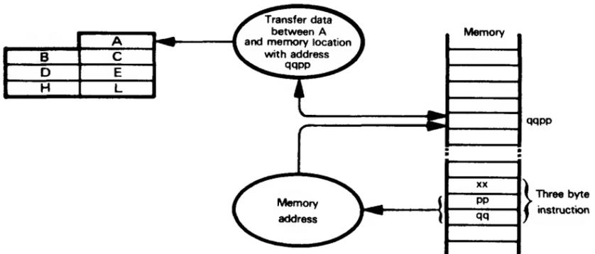
Since the Stack is part of the Read/Write memory, we must consider Push and Pop instructions as Memory Reference instructions. These instructions move two bytes of data between a register pair and the address in the Stack Pointer, i.e., current top-of-stack. The 8080A/8085 stack address is decremented with each Push and incremented with each Pop.
