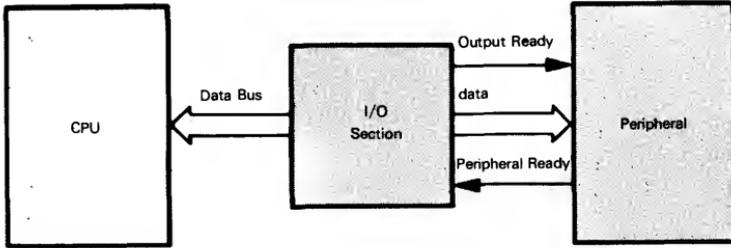
a) Peripheral provides Peripheral Ready signal to computer I/O section.
