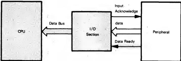
b) CPU reads Data Ready signal from I/O section (this may be a hardware, e.g., interrupt connection).
