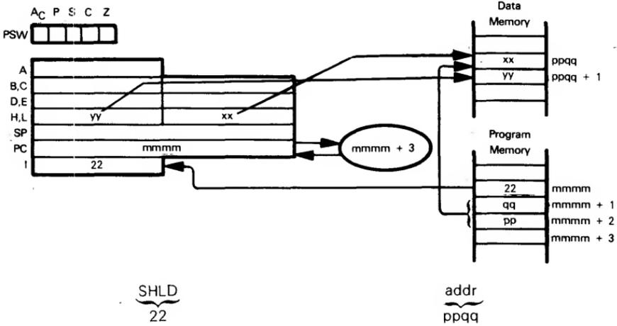
The second and third object code bytes provide the memory address of a data byte into which the L register contents are written. The H register contents are written into the next sequential data byte.
