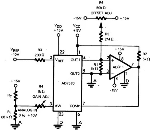
Note: If positive  $V_{REF}$  is used, the ANALOG INPUT range is 0 to  $-V_{REF}$ , and the COMPARATOR's (-) input should be connected to OUT1 (pin 4) of the AD7570.
