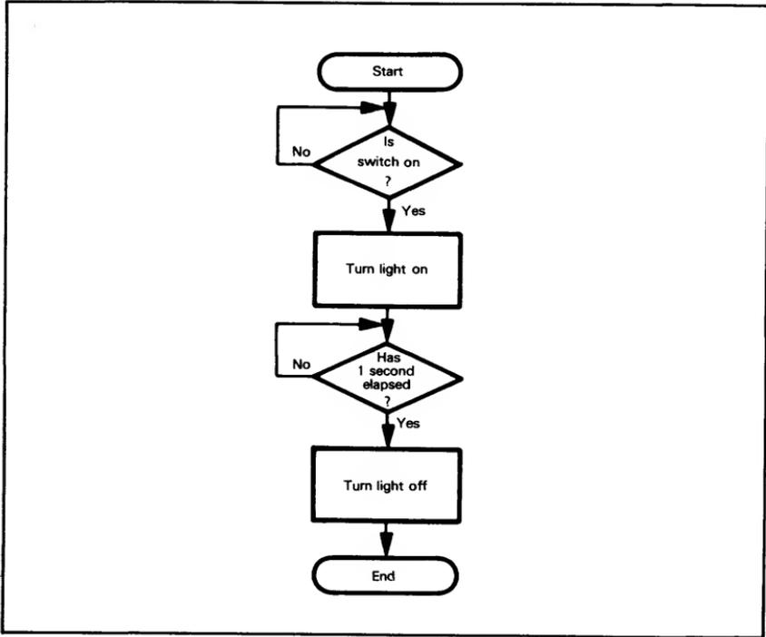
Figure 13-8. Flowchart Of One-Second Response To A Switch
