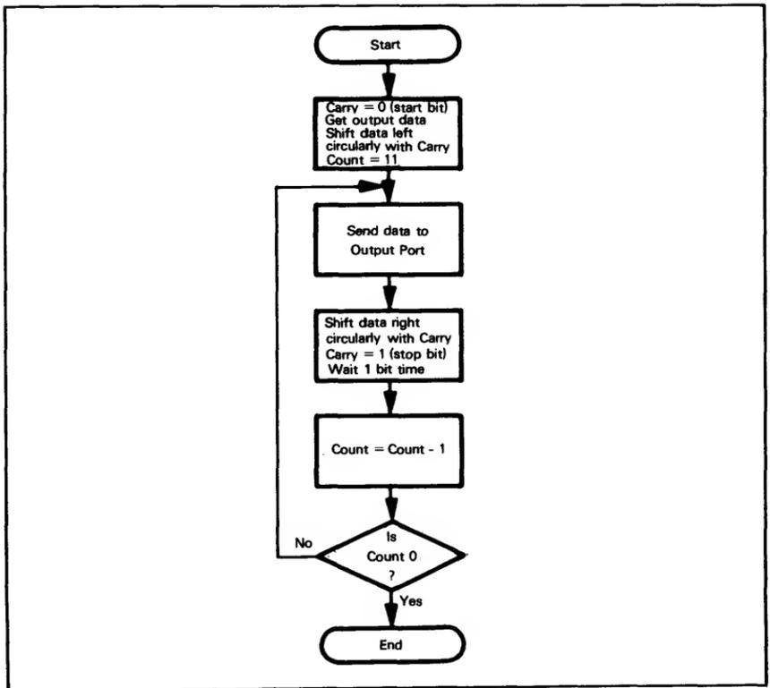
Figure 11-29. Flowchart For Transmit Procedure
