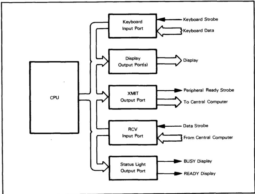
Figure 13-4. Block Diagram Of A Verification Terminal
