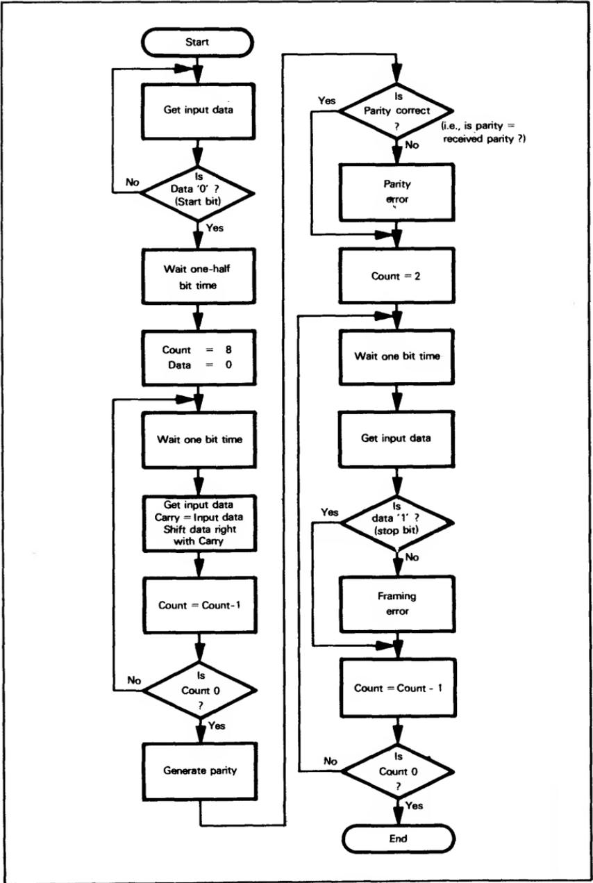
Figure 11-28. Flowchart For Receive Procedure
