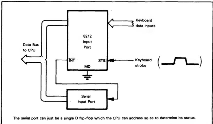
Figure 11-19. I/O Interface For An Encoded Keyboard
