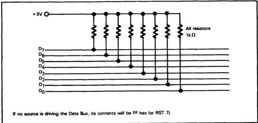
Figure 12-1. Using Pullup Resistors to Form the RST 7 Instruction
