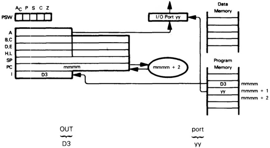
Output the contents of the Accumulator to the I/O port identified by the second OUT instruction object code byte.
