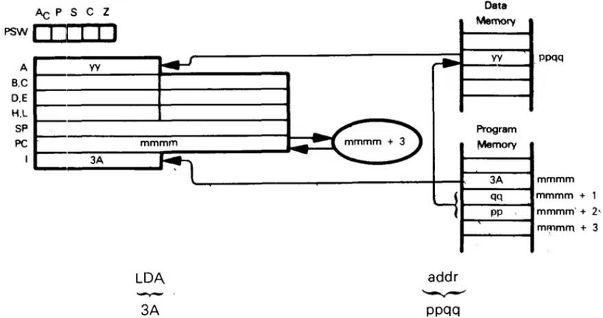
Load into the Accumulator the contents of the memory byte addressed directly by the second and third bytes of the LDA instruction object code.
