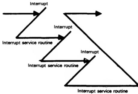
By inhibiting interrupts for one more instruction following execution of EI, the 8080 CPU insures that the RET instruction gets executed in the sequence:
