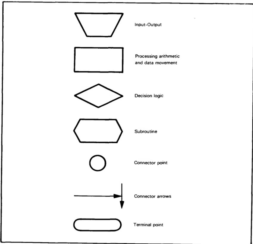
Figure 13-7. Standard Flow Diagram Symbols
