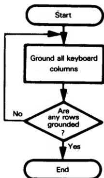
Key closures are identified by grounding all the keyboard columns and then checking for grounded rows (i.e., column-to-row switch closures). Note that the program does not assume any values for the unused input bits; instead, it masks off the bits attached to the keyboard rows with a logical AND instruction.
