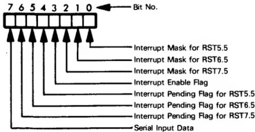
Bits 0, 1 and 2 are used to mask interrupts RST5.5, RST6.5 and RST7.5. If the bit corresponding to a particular RST is a 1, the RST is disabled. For example, if a RIM instruction results in 1A<sub>16</sub> being loaded in the Accumulator, this is what happens:
