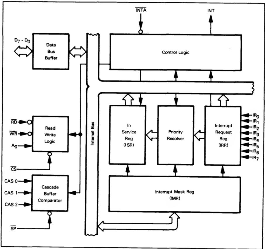
Figure 12-7. The 8259 Programmable Interrupt Controller
