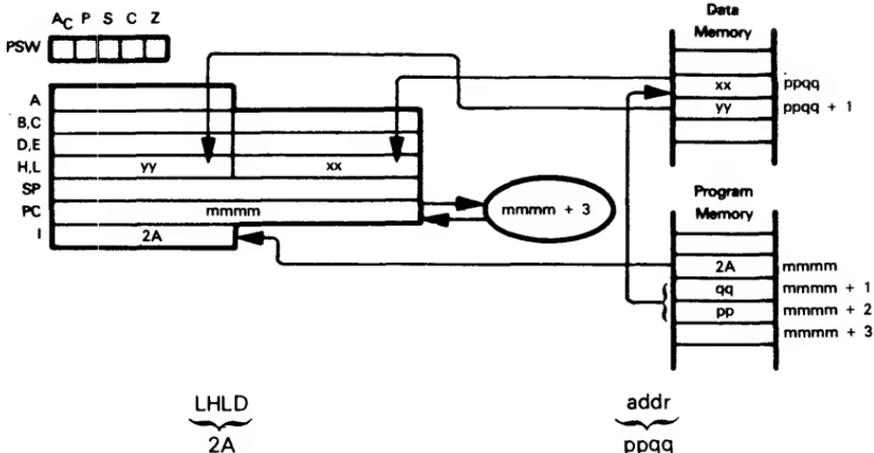
The second and third object code bytes provide the memory address of a data byte, the contents of which will be loaded into the L register. The contents of the next sequential data byte is loaded into the H register.
