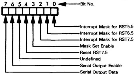
The interrupt mask function is only performed if the Mask Set Enable bit is 1. For example, if  $0F_{16}$  is held in the Accumulator and the SIM instruction is performed, 1 will be sent to the interrupt mask for all three RSTs. If, however,  $07_{16}$  was held in the Accumulator, the interrupt masks would not be affected.
