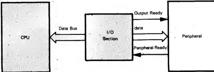
b) CPU reads Peripheral Ready signal from I/O section (this may be a hardware, e.g., interrupt connection).
