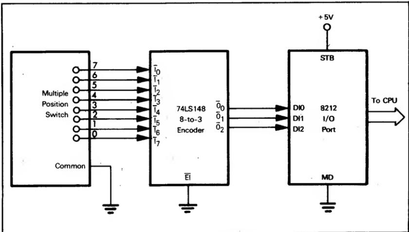
Figure 11-11. A Multiple-Position Switch With An Encoder
