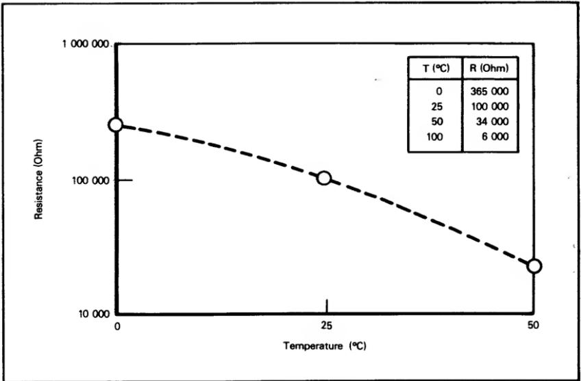
Figure 16-4. Thermistor Characteristics
