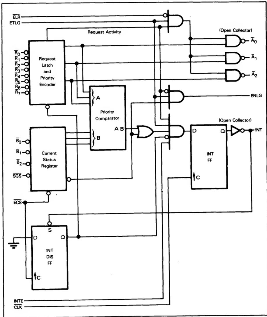
Figure 12-5. The 8214 Priority Interrupt Control Unit
