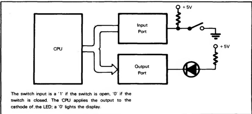
Figure 13-2. The Switch And Light System
