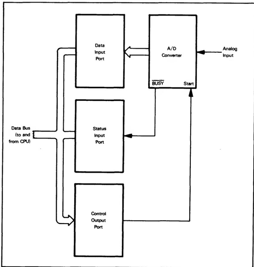
Figure 11-26. Interface For An 8-Bit Analog-To-Digital Converter
