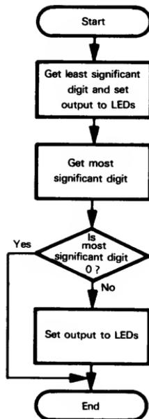
We remove the least significant digit by masking and set the bit which turns on the displays with a logical OR instruction. The result is saved in Register E.
