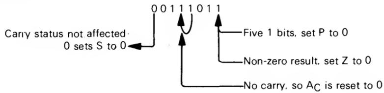
The contents of a read/write memory byte may also be incremented:
