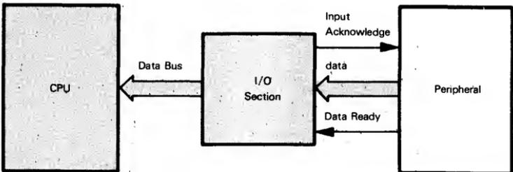
c) CPU reads data from I/O section.
