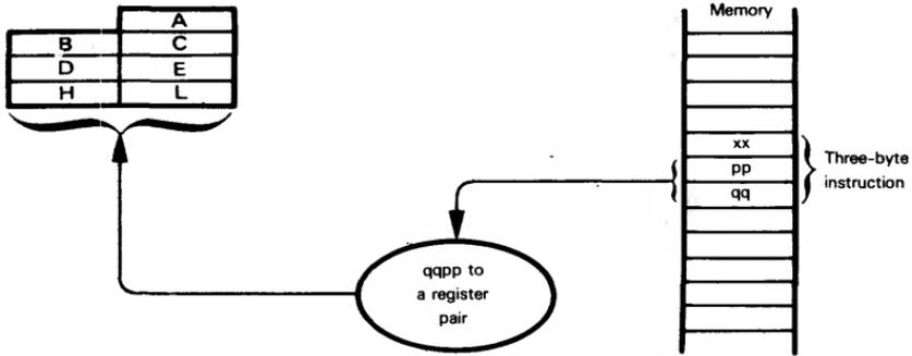
All 8080A and 8085 Jump instructions use absolute, direct addressing; that is to say, all Jump instructions are three bytes long, with the second and third bytes containing the address of the memory location from which the processor will fetch the next instruction to be executed.
