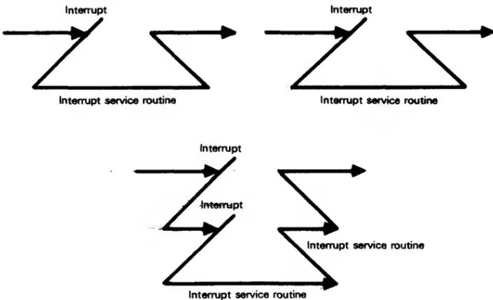
If interrupts are processed serially, then priority arbitration will apply only during the acknowledge process.
