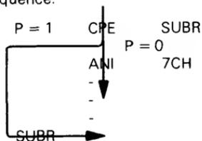
After the CPE instruction has executed, if the Parity status does not equal 1 the ANI instruction will be executed. If the Parity status does equal 1, the address of the ANI instruction is saved at the top of the stack. The Stack Pointer is decremented by 2. The instruction labeled SUBR will be executed next.
