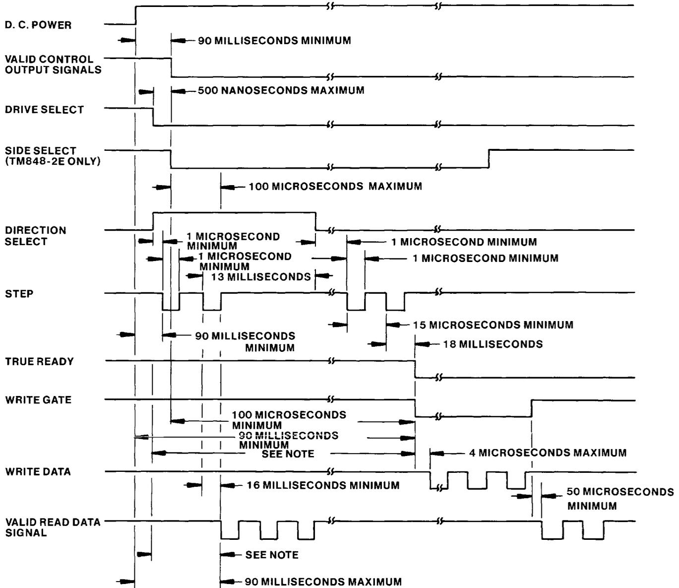
NOTE: 150 MILLISECONDS, MINIMUM, DELAY MUST BE INTRODUCED AFTER DRIVE SELECT TO ALLOW TIME FOR THE D. C. MOTOR TO REACH 360 RPM OR THE OPTIONAL TRUE READY LINE MUST BE MONITORED.
