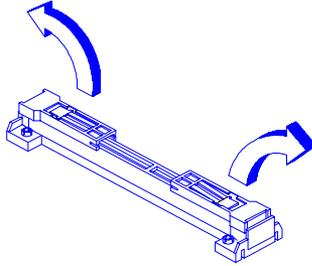
2. Place the universal retention mechanism over the CPU connector on the system board and press it until it clicks into place.
