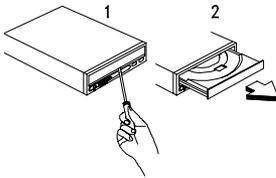
Locate the bottom edge of the disc tray. Gently pry the disk tray open with a screwdriver. When the disc tray opens, simply remove the disc from the CD-ROM drive.
