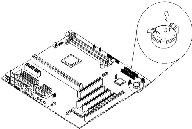
**IMPORTANT:** Make sure to insert the battery with the positive side facing up. A plus(+) sign indicates the positive side.
