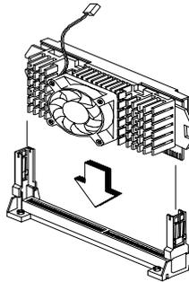
**CAUTION:** The electrical contacts of the Pentium III module are slotted in such a way that the module only fits in one direction. Make sure that the module groove matches the one on the processor socket.
