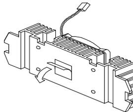
5. Align the four tabs of the fastener with the four holes on the Celeron processor.
