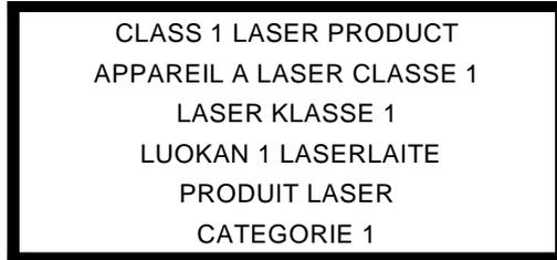
The CD/DVD-ROM drive is certified in the U.S. to conform to the requirements of the Department of Health and Human Services 21 Code of Federal Regulations (DHHS 21 CFR) Subchapter J for Class 1 laser products.
