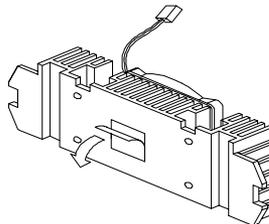
5. Align the four tabs of the fastener with the four holes on the Celeron processor.
