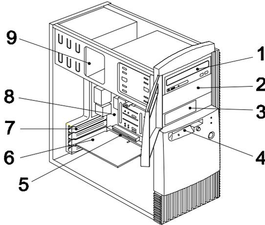
This computer system has four bays that can hold 5.25-inch and 3.5-inch drives. Additional devices can be installed in the empty bays.
