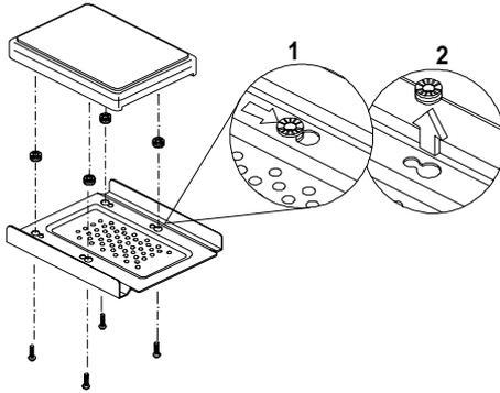
**ATTENTION:** When installing the hard disk drive, the cushion rings and shoulder screws must be used to secure the hard disk to the tray.
