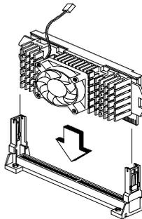
**CAUTION:** The electrical contacts of the Pentium III module are slotted in such a way that the module only fits in one direction. Make sure that the module groove matches the one on the processor socket.
