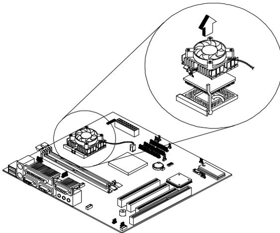
**NOTE:** Installing the processor
