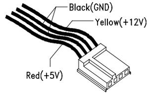
**006 - ARE THE VOLTAGES CORRECT AND DOES THE FAN RUN? (YES, READ AHEAD. NO, GO TO STEP 009.)**
