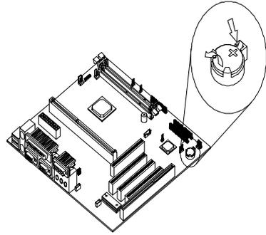
**IMPORTANT:** Make sure to insert the battery with the positive side facing up. A plus(+) sign indicates the positive side.
