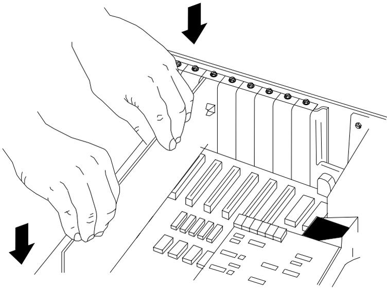
4. Install the co-processor adapter's mounting screw.
