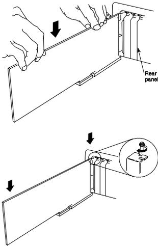
12. Align the slot in the card-retaining bracket with the hole in the rear panel of the system unit.
