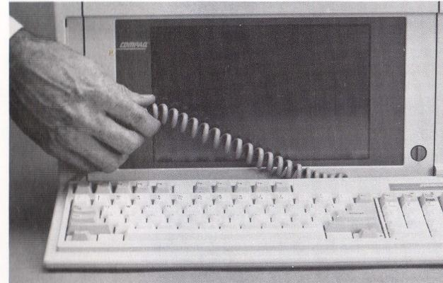
Figure 2-4. Lifting the Keyboard Cord Out of the Cable Storage Tray.
