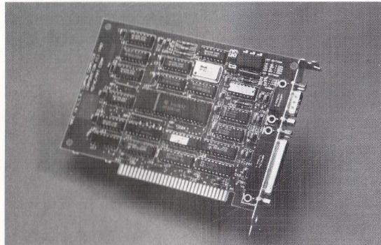
Figure 8-16. Asynchronous Communications/Parallel Printer Board.
