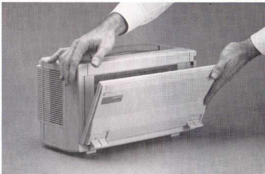
Figure 4-2. Securing the Keyboard.
