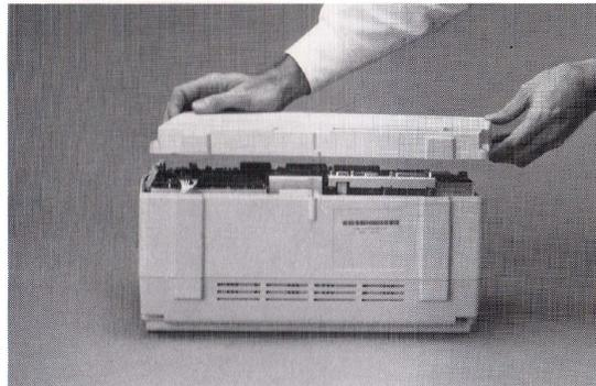
Figure 7-5. Replacing the Rear Panel.
