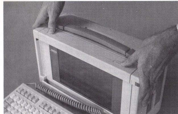
Figure 2-5. Releasing the Plasma Display from the Locked Position.
