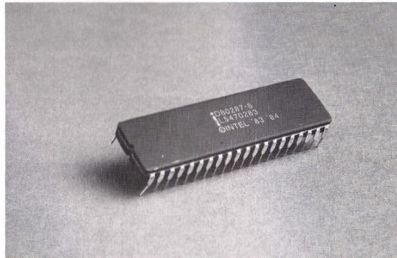
Figure 8-13. 8-MHz 80287 Coprocessor.
