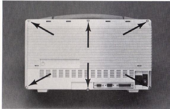
Figure 7-1. Location of Rear Panel Screws and Washers.
