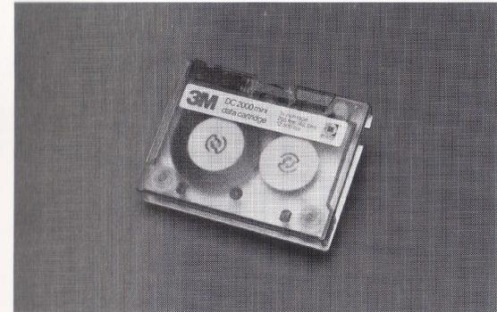
Figure 8-4. DC-2000 Tape Cartridge.
