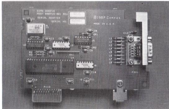
Figure 8-17. Second Asynchronous Communications Interface Board.
