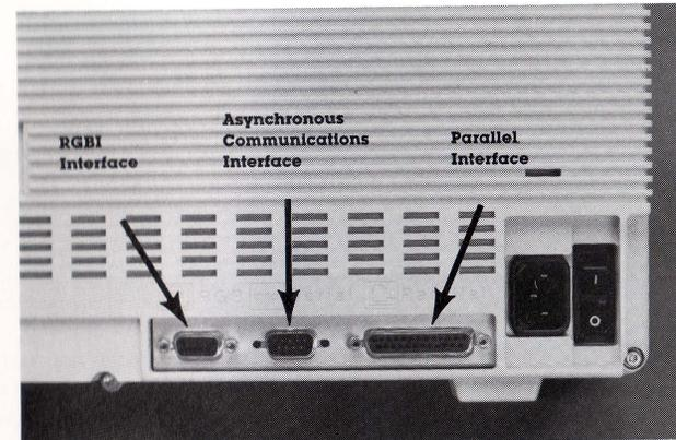
Figure 2-10. Interface Connectors on the Back of the COMPAQ PORTABLE III Personal Computer.
