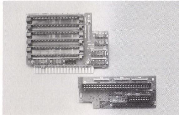
Figure 8-12. Memory Expansion Board and 16-Bit Memory/Modem Interface Board.
