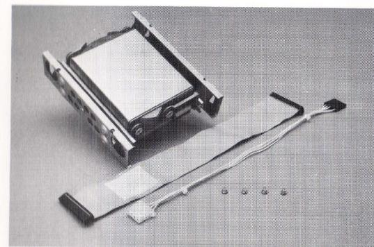
Figure 8-1. 20-Megabyte Fixed Disk Drive Option Kit.
