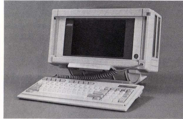
Figure 1-1. COMPAQ PORTABLE III Personal Computer.
