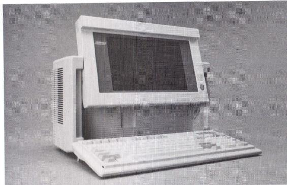
Figure 2-6. Plasma Display in an Upward Position.
