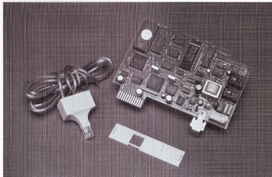
Figure 8-7. COMPAQ 2400 Baud Internal Modem Option Kit.
