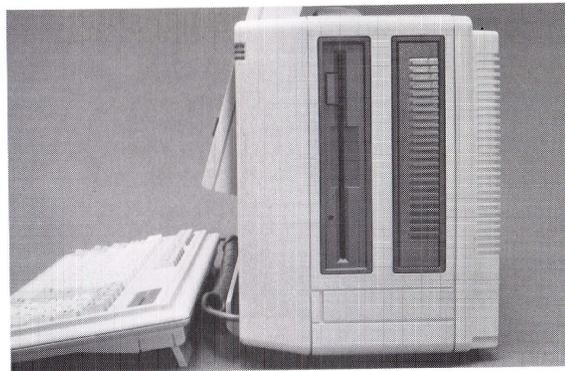
Figure 2-7. Drive Positions on the COMPAQ PORTABLE III Personal Computer.
