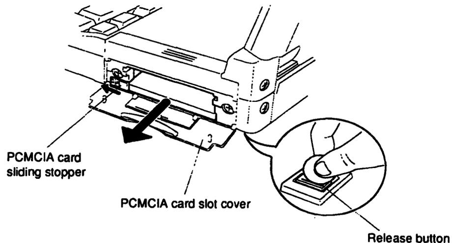
*Figure 4-3 Removing the PCMCIA Card*
