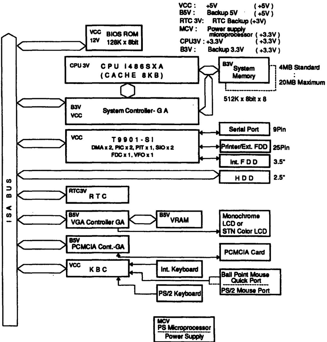
Figure 1-3 T1900/T1900C System Board Block Diagram
