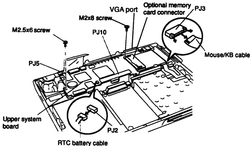
*Figure 4-18 Removing the Upper System Board*
