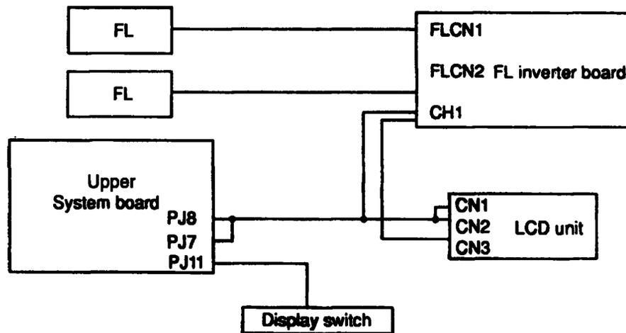
*Figure 2-4 T1900C Display Connections*
