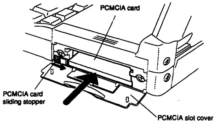
*Figure 4-4 Installing the Optional PCMCIA Card*
