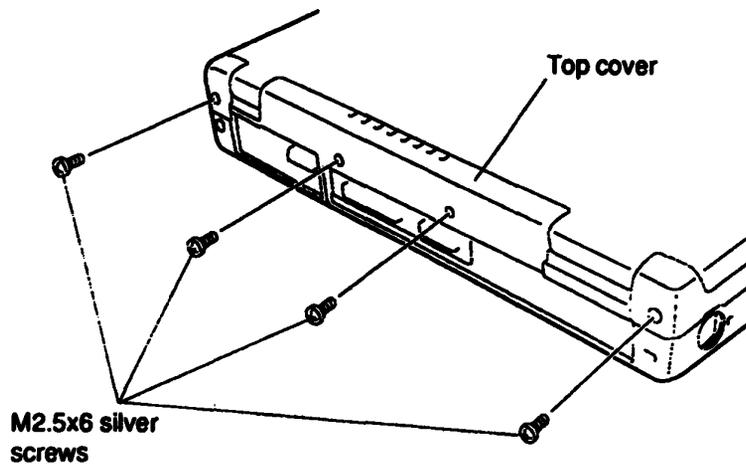
*Figure 4-5 Removing Top Cover Screws*
