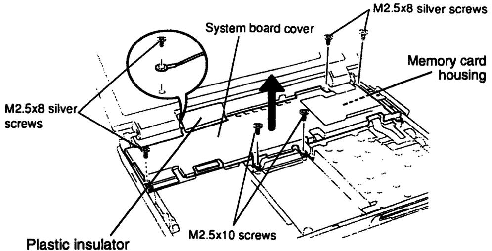
*Figure 4-16 Removing the System Board Cover*
