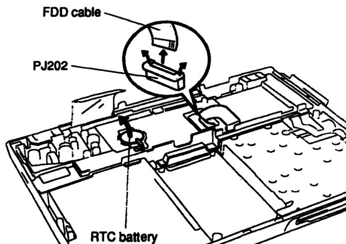
*Figure 4-19 Removing the RTC Battery and FDD Cable*
