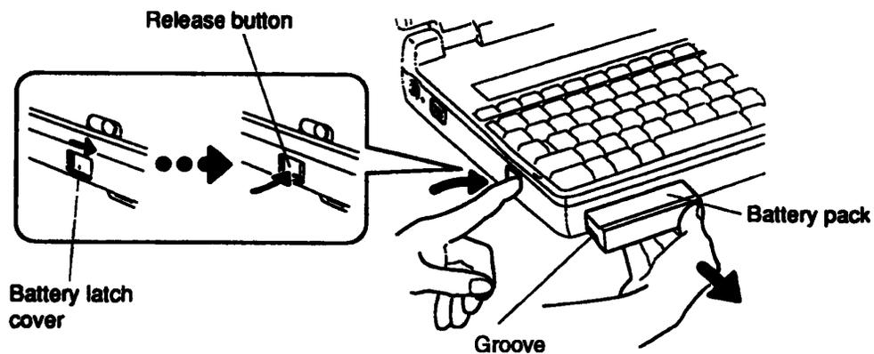
*Figure 4-1 Removing the Battery Pack*
