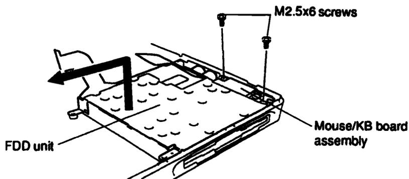
*Figure 4-23 Removing the FDD and Mouse/KB Board*
