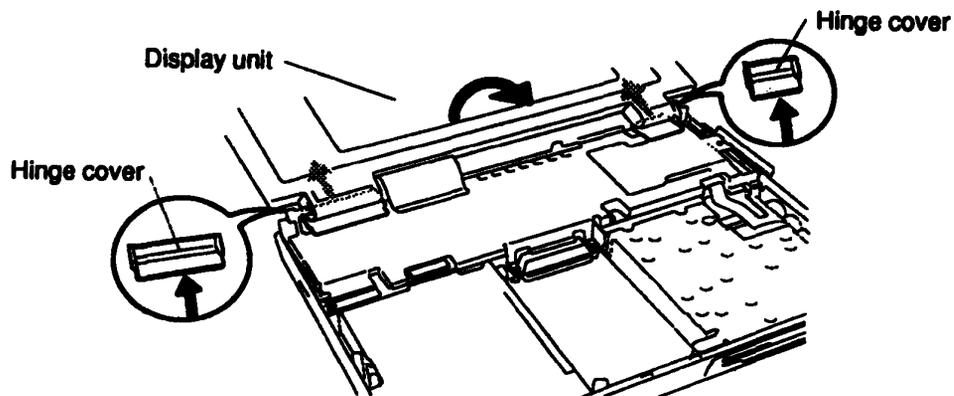
*Figure 4-15 Removing the Hinge Covers*
