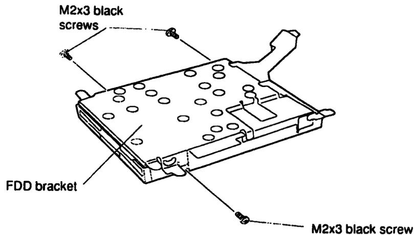
*Figure 4-25 Removing the FDD Bracket*
