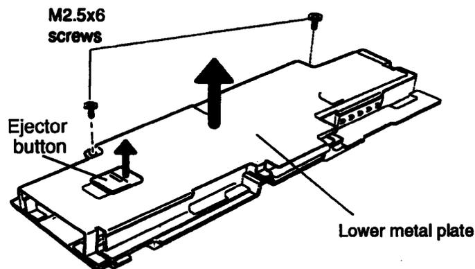
*Figure 4-21 Removing the Lower Metal Plate*
