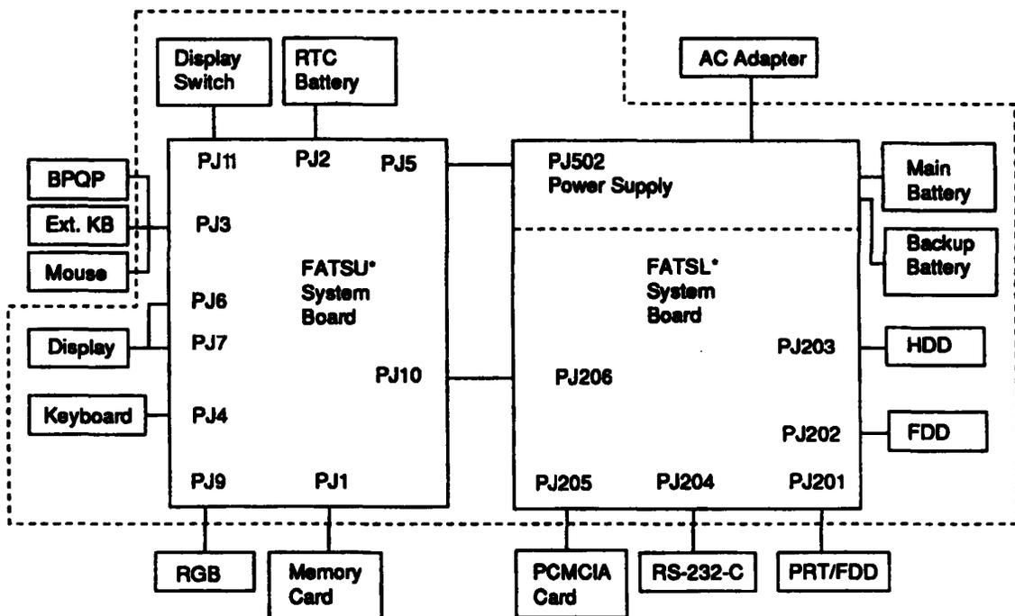
Figure 1-2 T1900/T1900C System Unit Configuration
