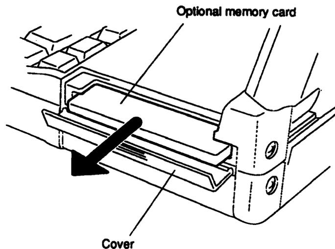
*Figure 4-2 Removing the Optional Memory Card*
