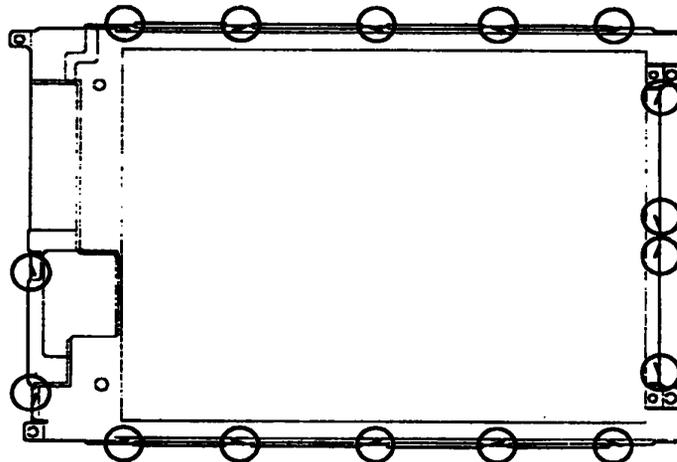
*Figure 4-29 Unbending the Color LCD Module Latches*
