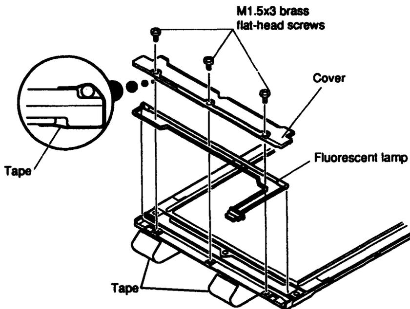
*Figure 4-35 Removing the Fluorescent Lamp*
