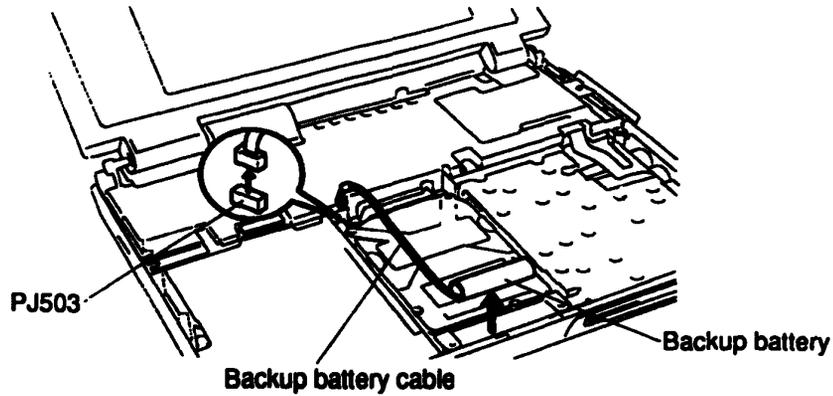
*Figure 4-10 Removing the Backup Battery*
