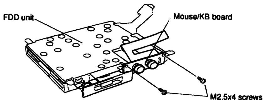
*Figure 4-24 Separating the FDD and Mouse/KB Board*
