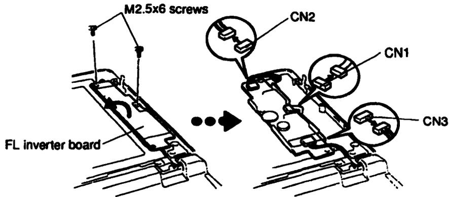
*Figure 4-27 Removing the FL Inverter Board*
