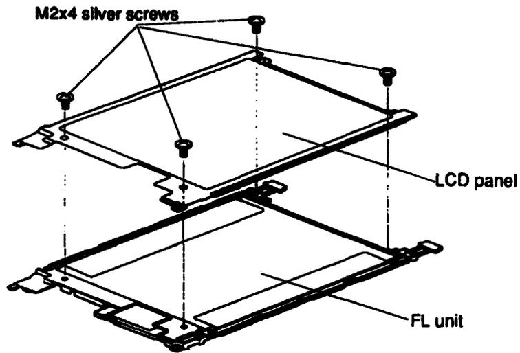
*Figure 4-30 Removing the FL Screws*
