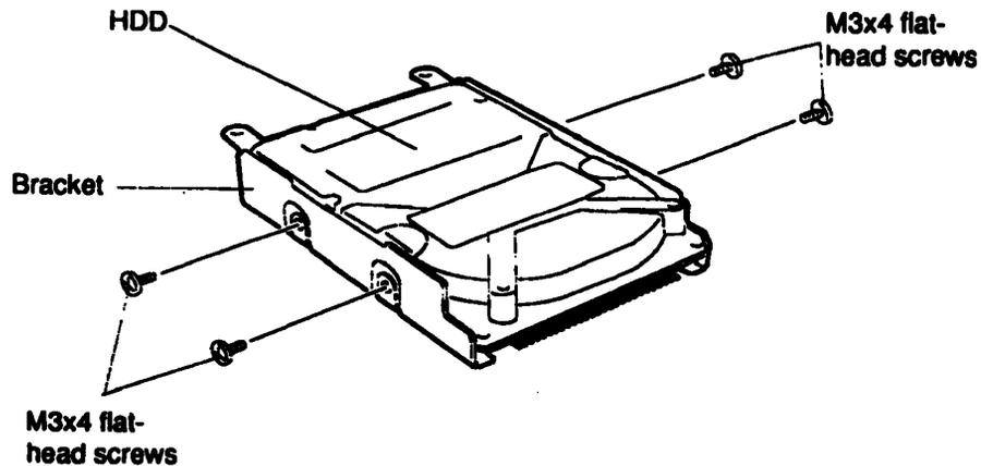
*Figure 4-12 Removing the Bracket from the HDD*
