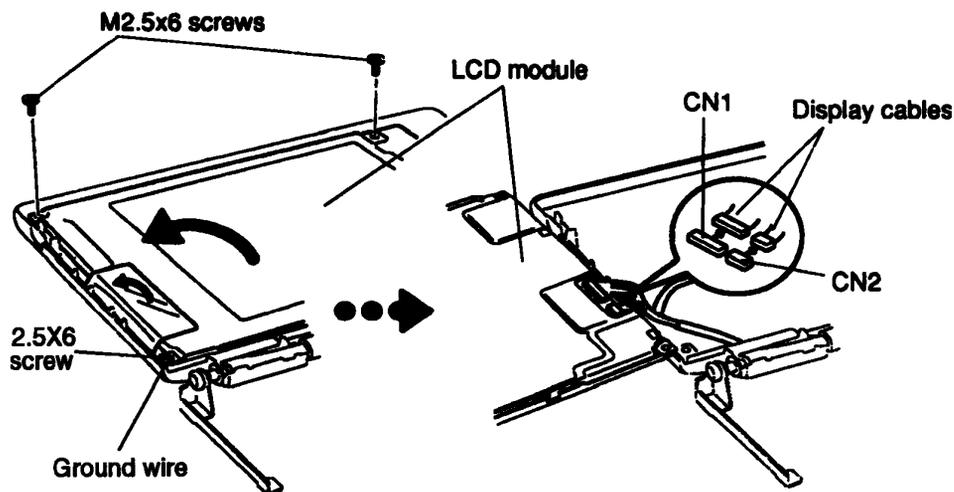
*Figure 4-34 Removing the LCD Module*
