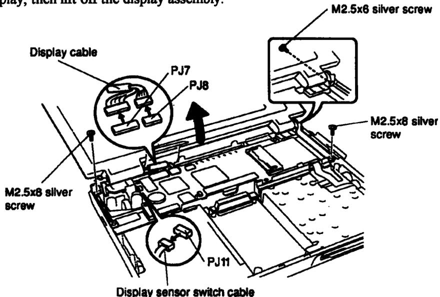
*Figure 4-17 Removing the Display Assembly*
