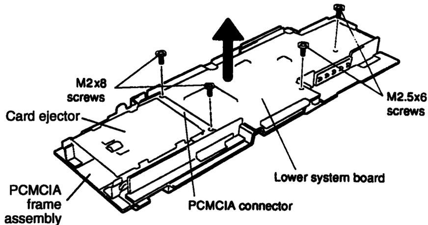
*Figure 4-22 Removing the Lower System Board*
