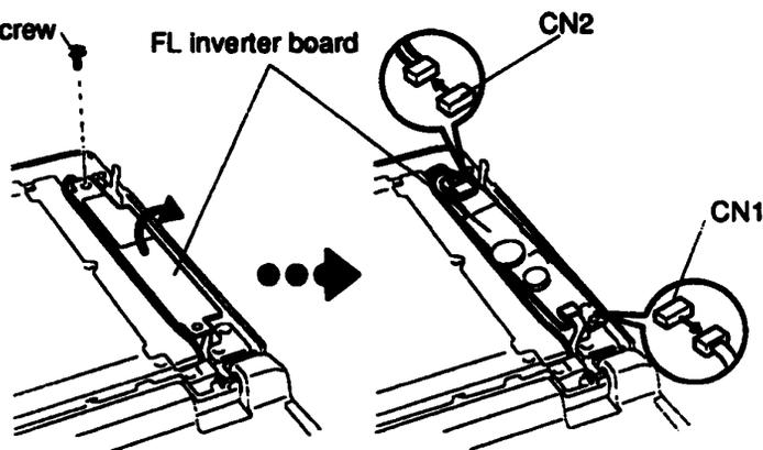
*Figure 4-33 Removing the FL Inverter Board*
