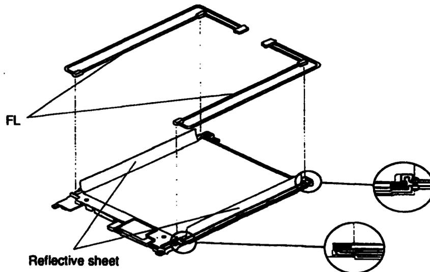
*Figure 4-31 Removing the FL*
