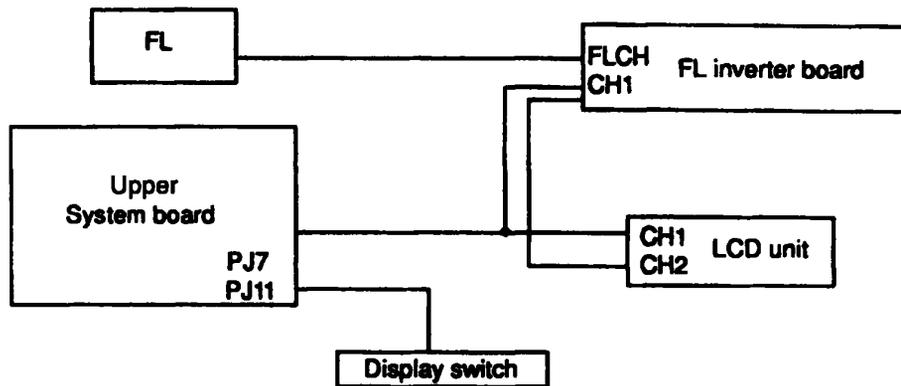
*Figure 2-3 T1900 Display Connections*
